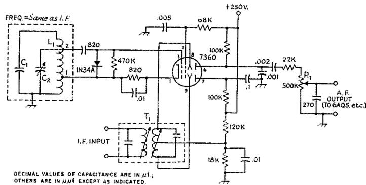
Fig. 6—Product detector circuit with self-excitation. The beat-frequency oscillator tuned circuit,  $C_1C_2L_1$ , should be high- $Q$  at the intermediate frequency used;  $C_2$  is for fine frequency adjustment. On  $L_1$ , tap 1 is at approximately
