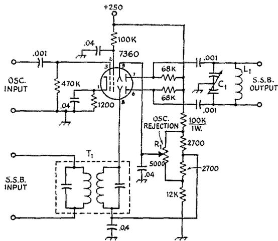
Fig. 4— Balanced mixer circuit with separate excitation. Capacitances are in  $\mu\text{f}$ .; fixed resistors are  $\frac{1}{2}$  watt except as indicated. Tuned-circuit constants depend on frequency; ordinary  $L/C$  ratios may be used for  $L_1C_1$  and in the s.s.b. input transformer,  $T_1$ .  $R_1$  is a linear-taper composition potentiometer.
