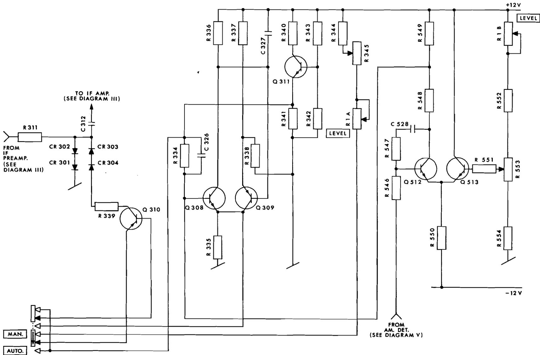
Fig. F1. IF attenuator and AGC amplifier.
