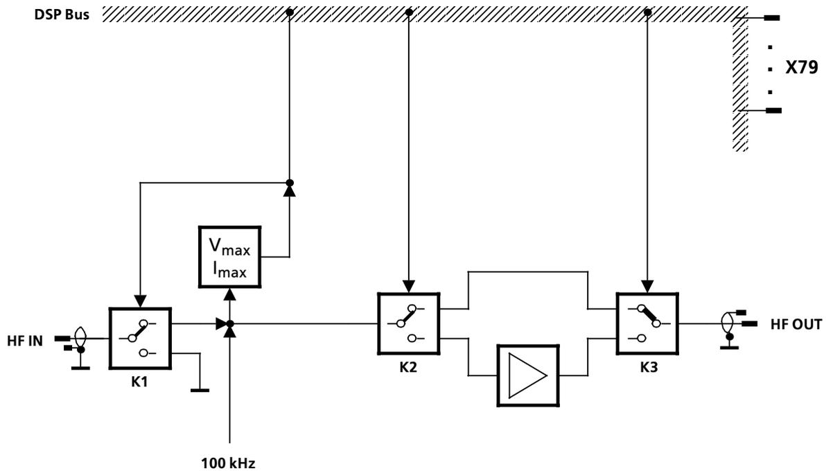
Fig. 1.13 IF / AF Processor (Preamplifier and Protective Circuit), Block Diagram
