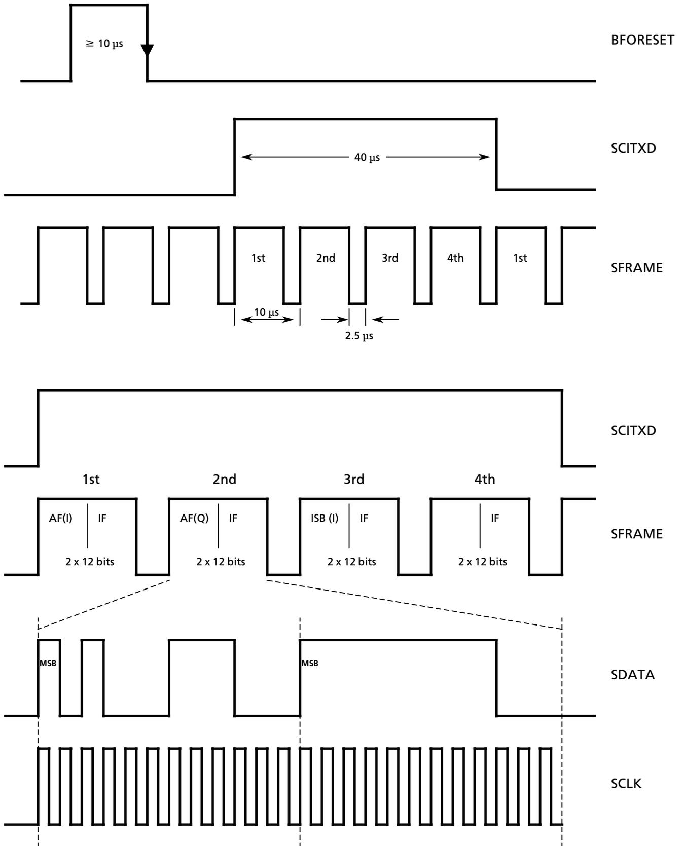
Fig. A2.1 Representation of Signals SFRAME, SCLK, SDATA, SCITxD and BFO Reset
