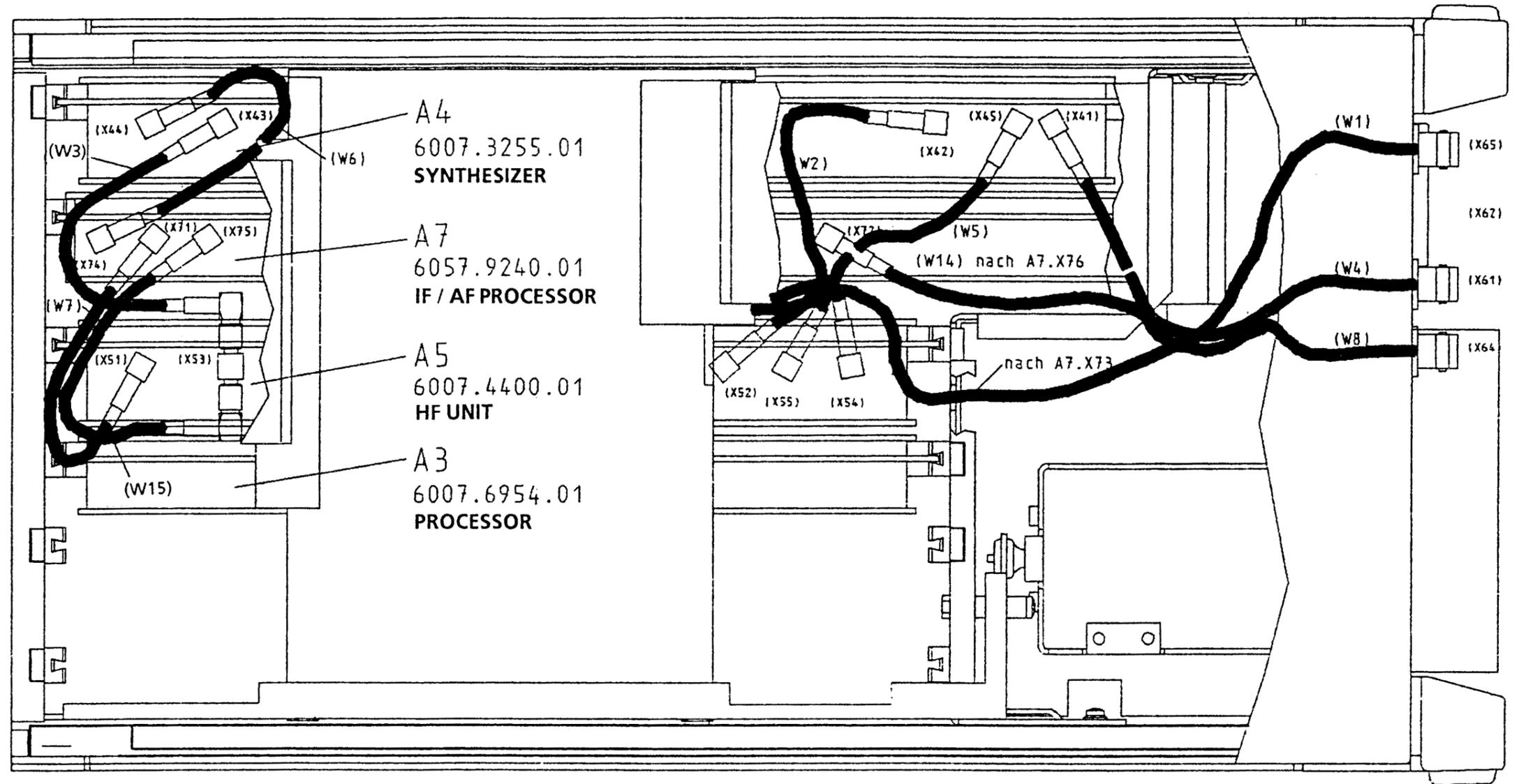
Fig. A1.7 Internal Cabling
