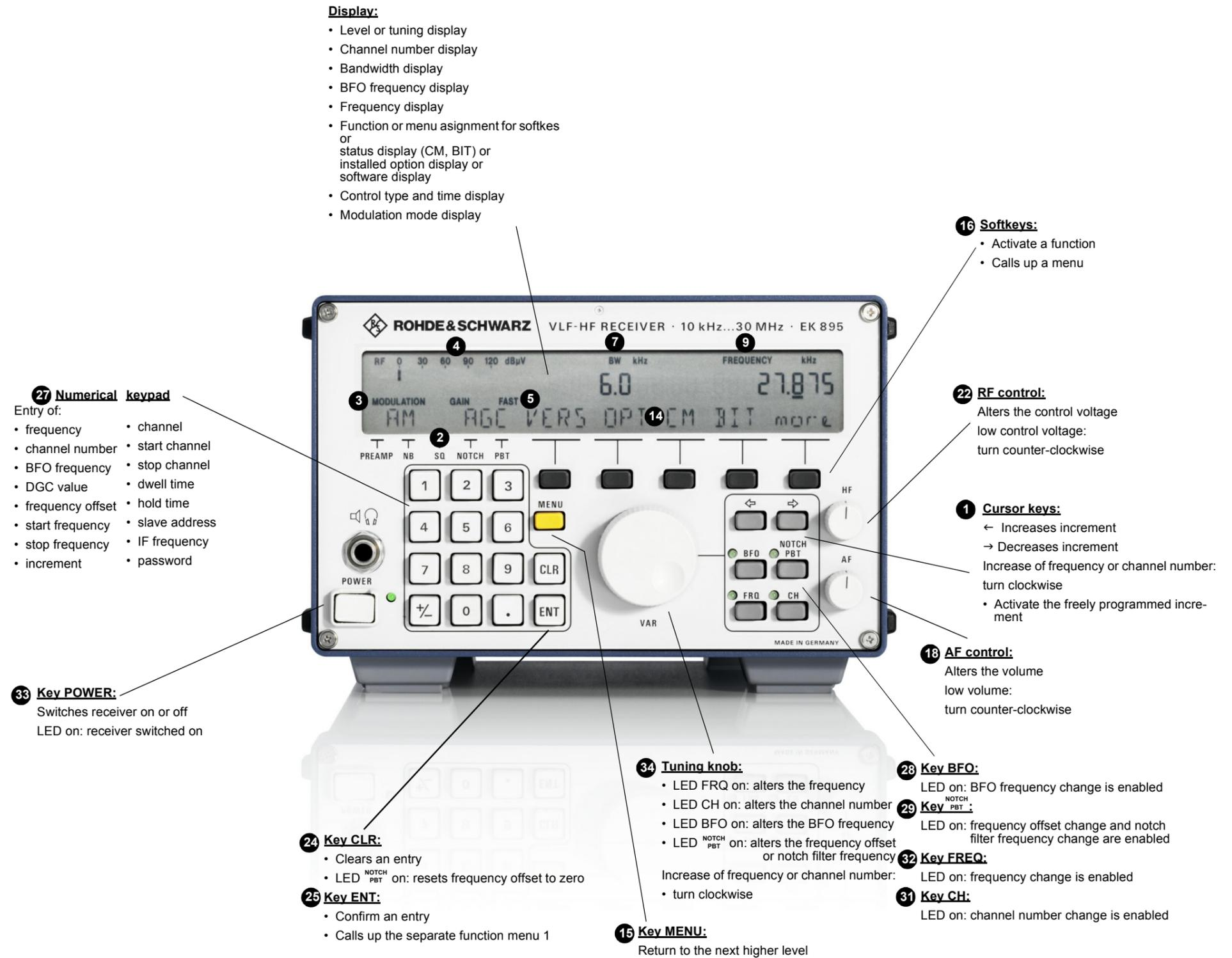
Fig. 3.2 Control and Display Elements of VLF-HF Receivers R&S EK 895 (Local)
