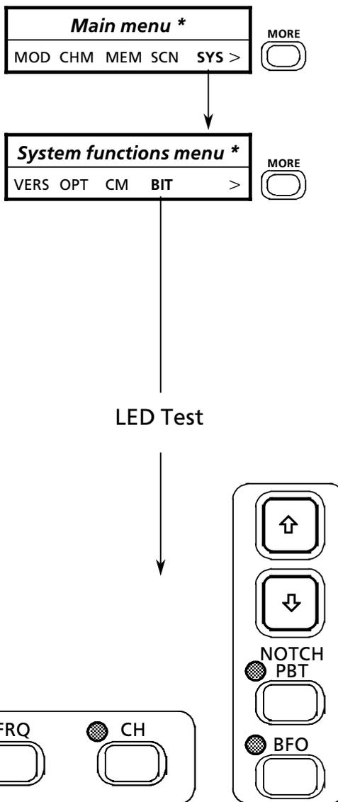
Via the LED test the function of LEDs FRQ, BFO, CH and PBT / NOTCH is checked.
