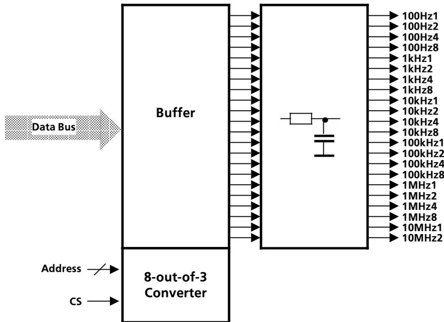
Fig. 1.15 BCD Interface R&S GC 890 (Option), Block Diagram
