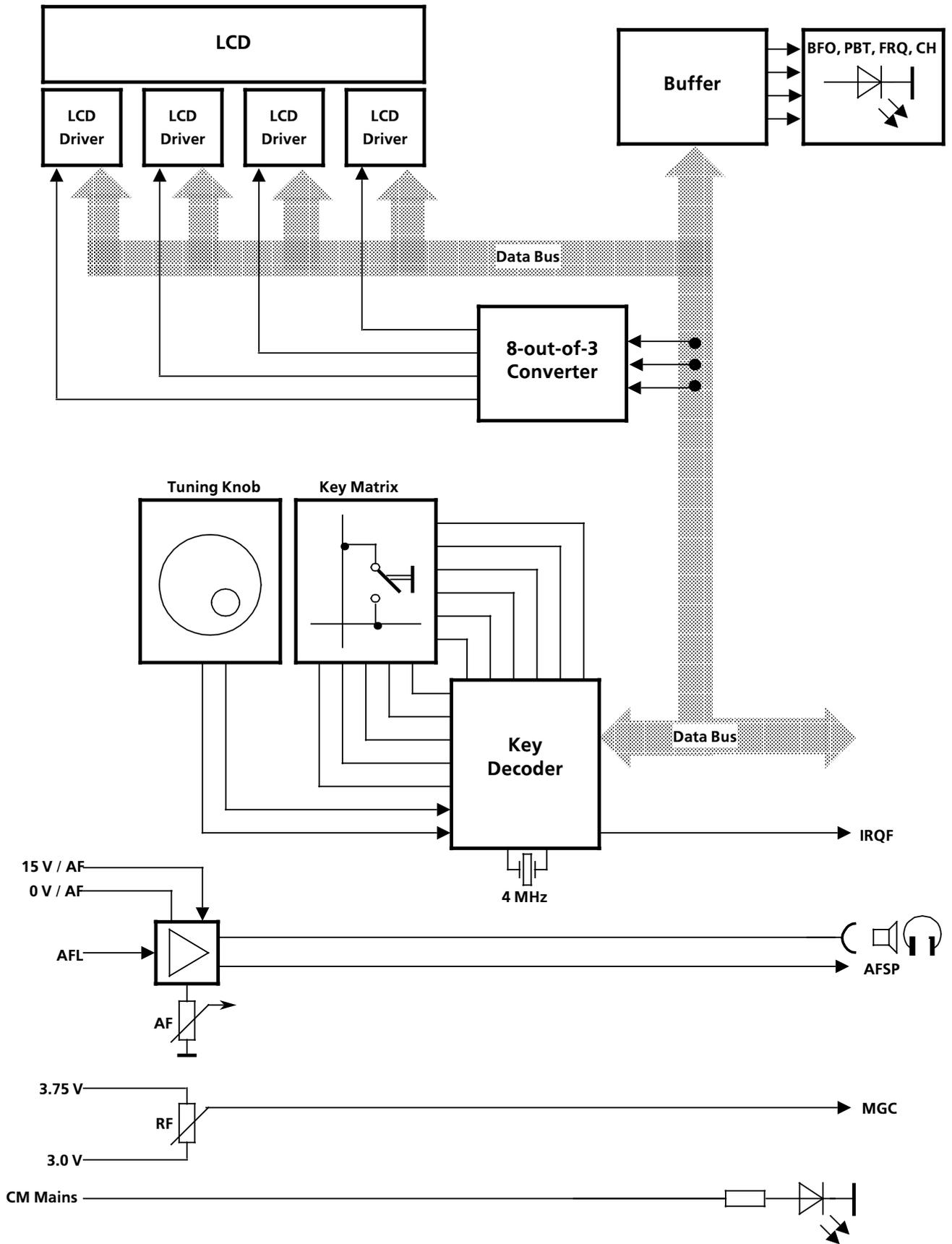
Fig. 1.6 Control Unit 2 "LOCAL" (R&S EK 895, Option 'Control Unit R&S GB 890'), Block Diagram
