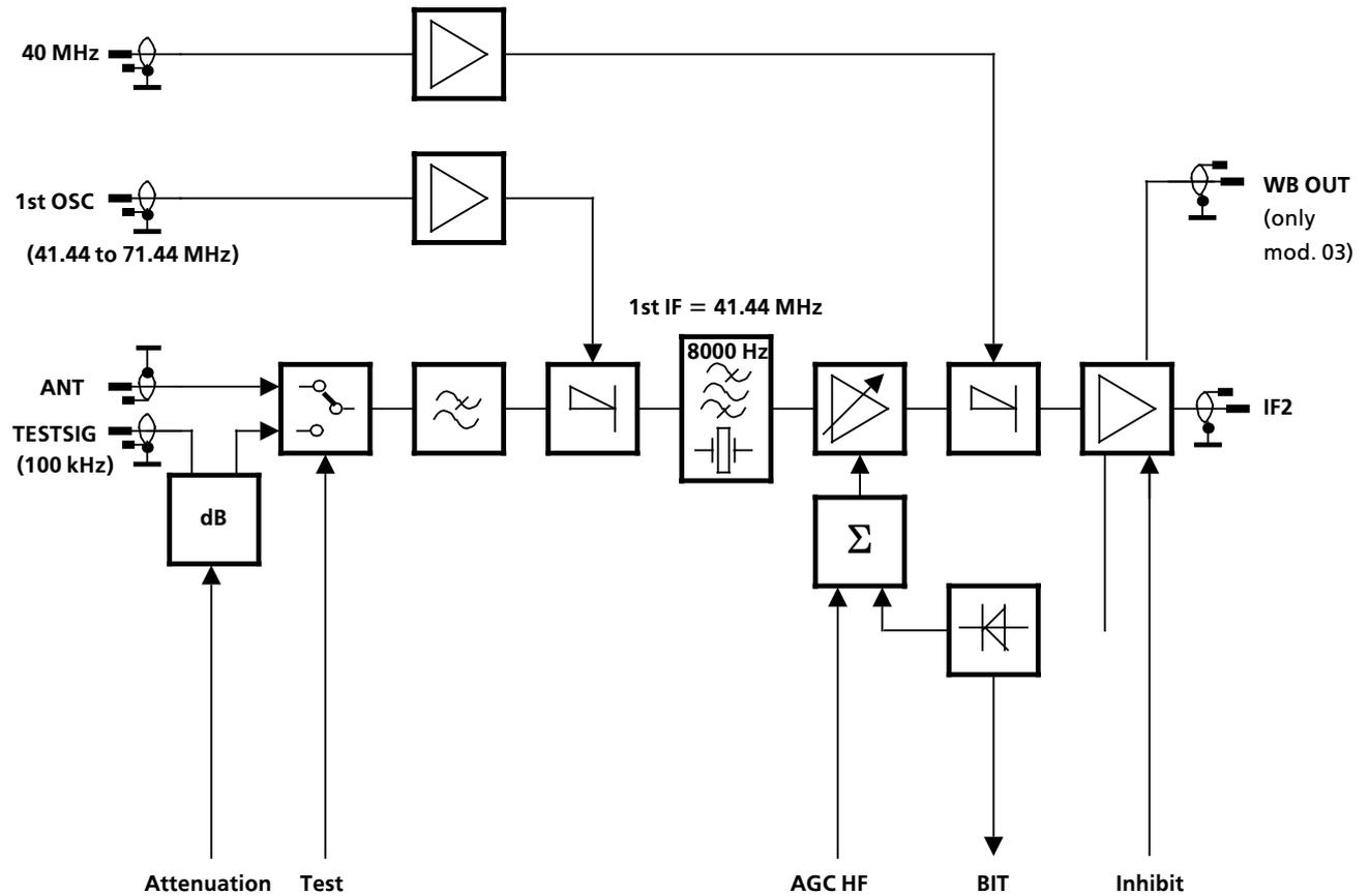
Fig. 1.10 HF Unit, Block Diagram
