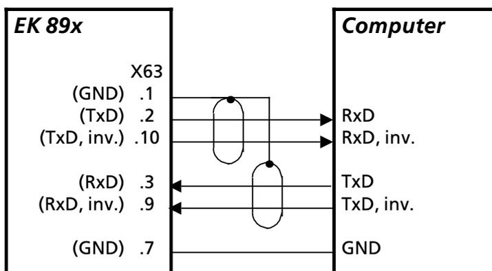
Fig. 2.16 Operating Mode: RS422 with XON-XOFF Handshake (S4 = 6 or 7; see A1.4)
