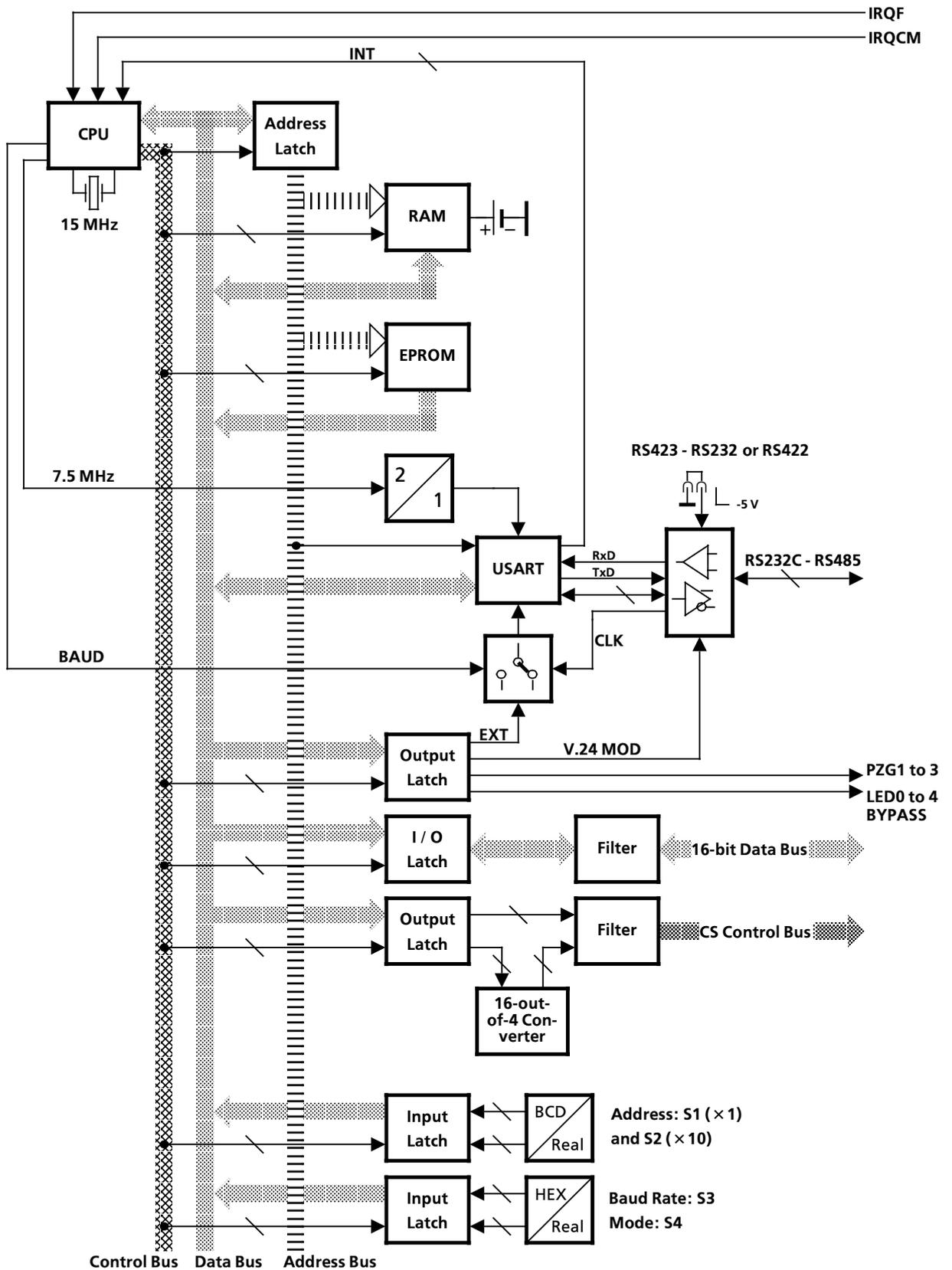
Fig. 1.8 Processor, Block Diagram
