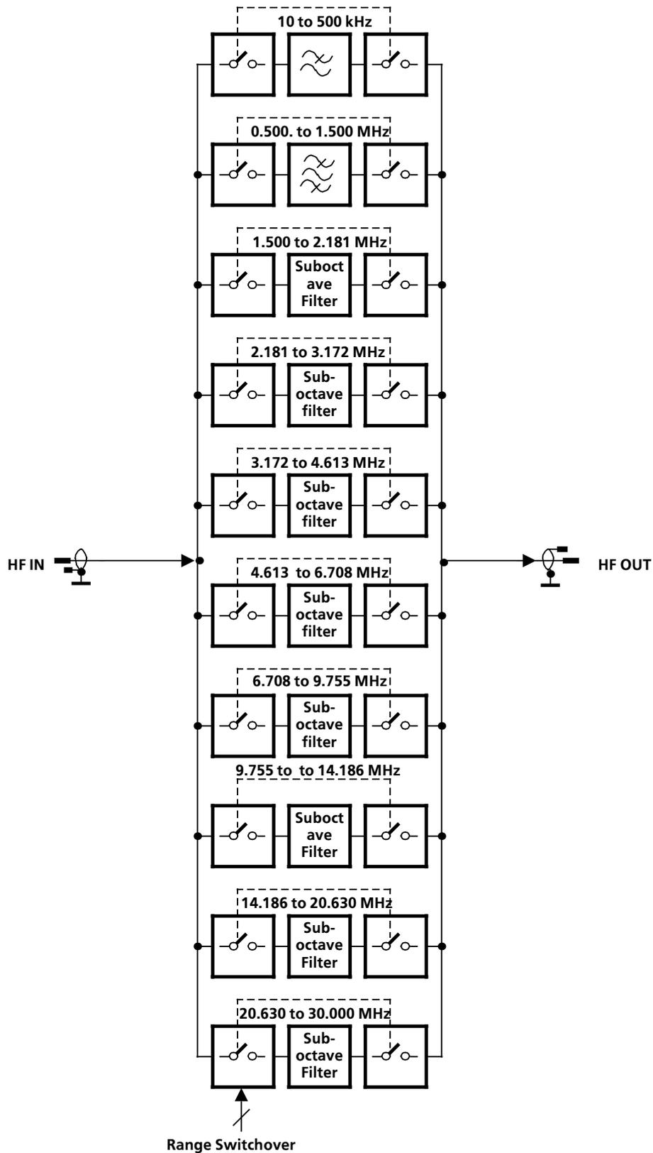
Fig. 1.14 Preselection R&S FK 890H1 (Option), Block Diagram
