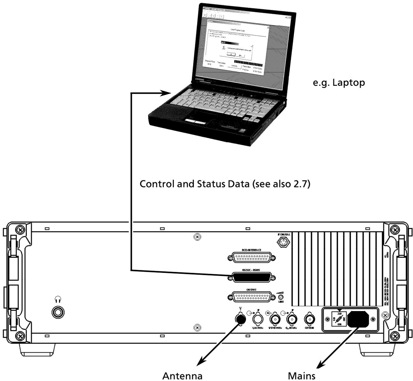
Fig. 2.10 Connection of a PC to VLF-HF Receiver EK 896
