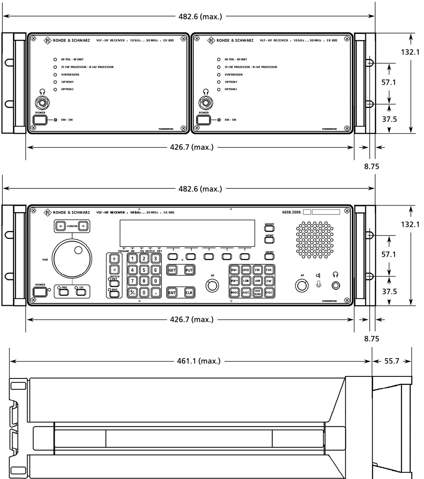
Fig. 2.24 Installation Drawing
