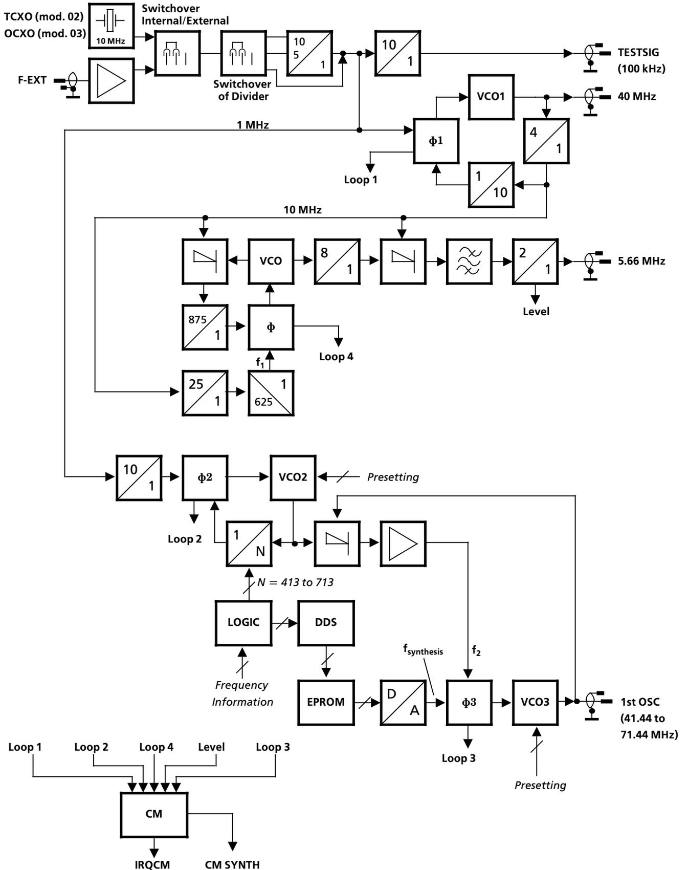
Fig. 1.9 Synthesizer, Block Diagram
