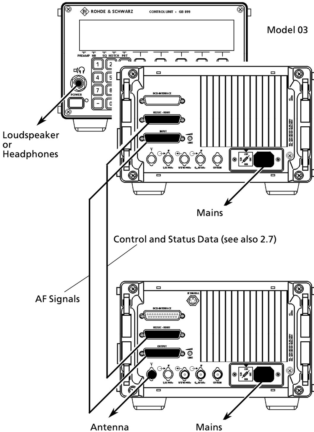
Fig. 2.8 Connection of Control Unit GB 899 to VLF-HF Receiver EK 895
