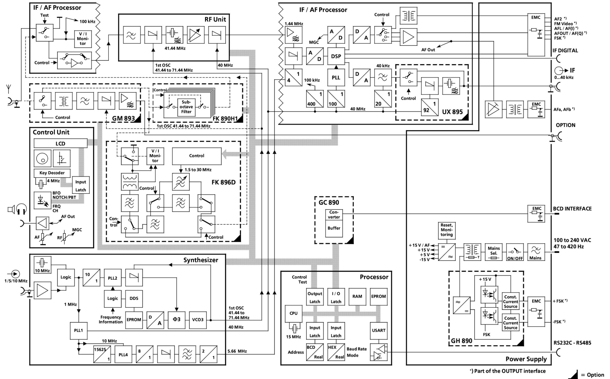
Fig. 1.21 VLF-HF Receivers R&S EK 896, Block Diagram
