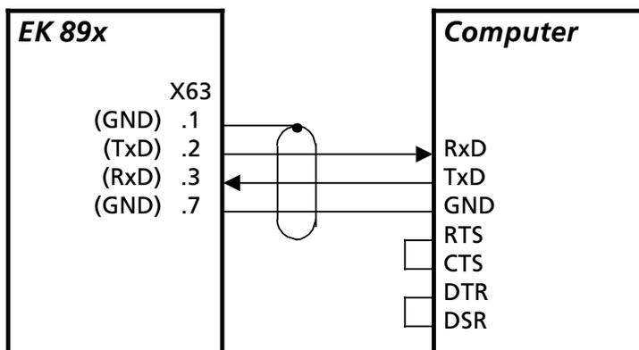
Fig. 2.14 Operating Mode: RS232 with XON-XOFF Handshake (S4 = 0, 1, 2 or 3; see A1.4)
