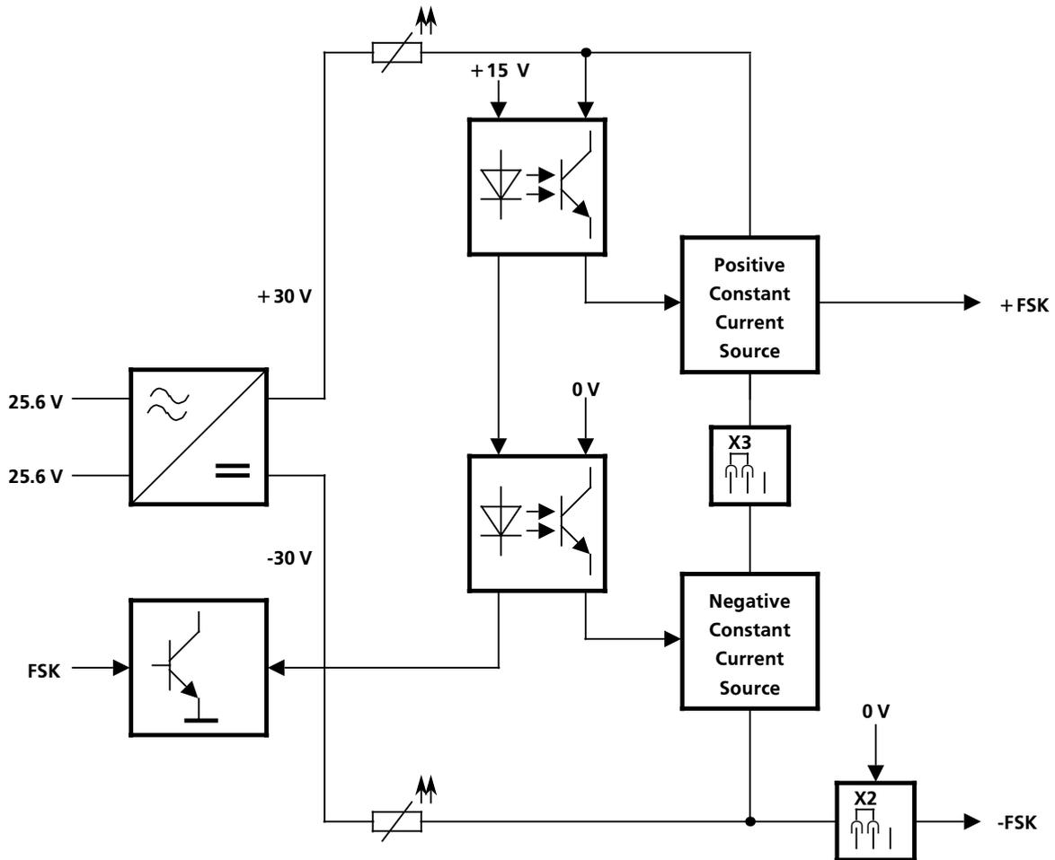
Fig. 1.16 TTY Line Current Source R&S GH 890 (Option), Block Diagram
