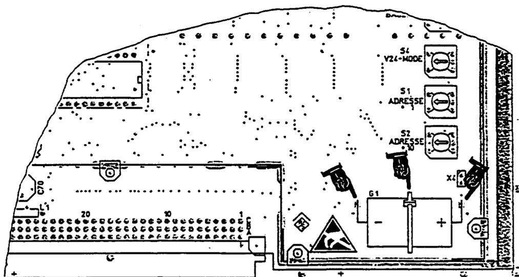
**Fig. 4.5 Location of Back-up Battery**
