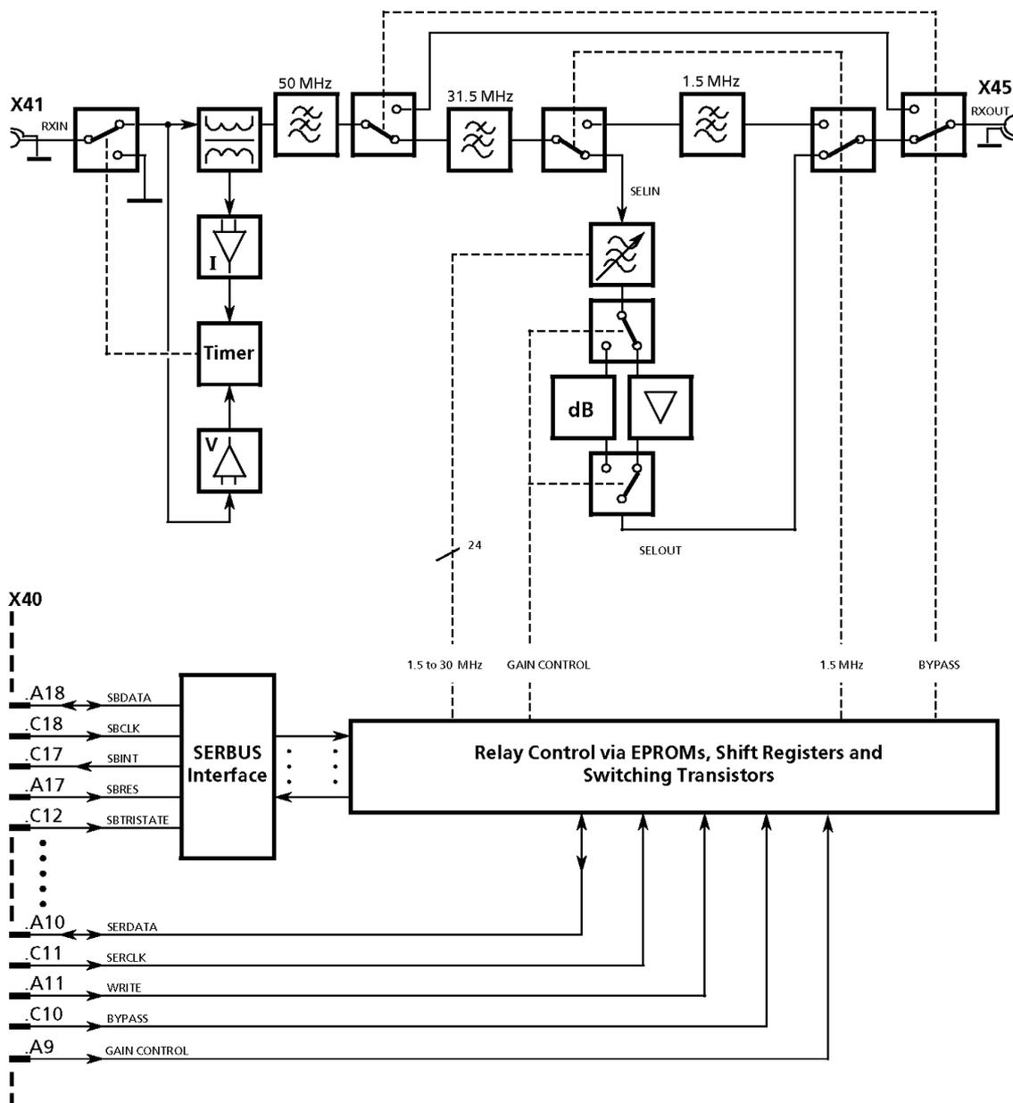
Fig. 1.19 Digitally Tuned RF Selector R&S FK 896D
