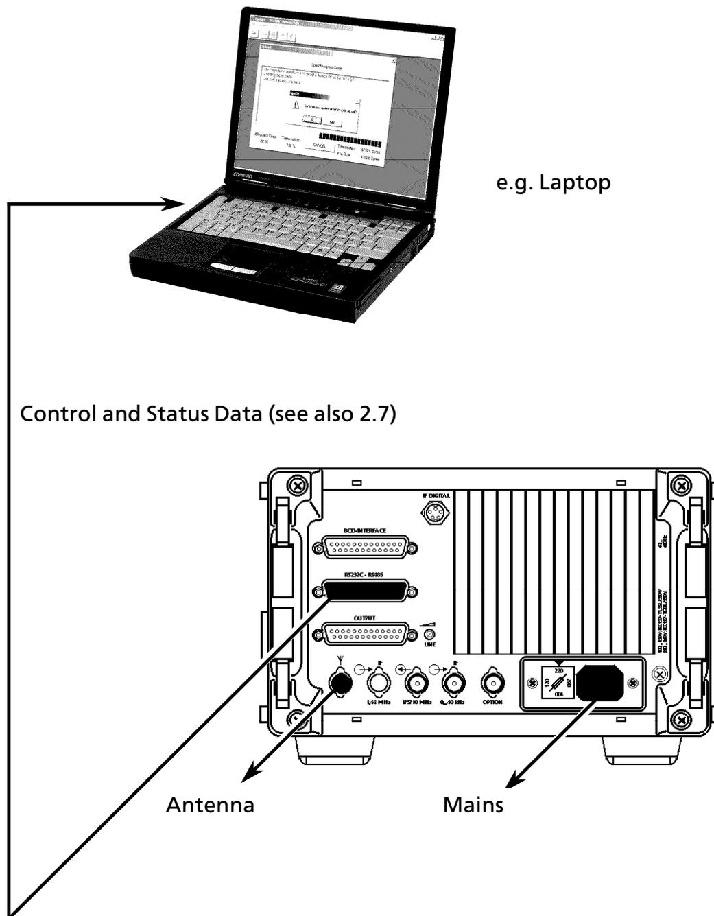
Fig. 2.9 Connection of a PC to VLF-HF Receiver EK 895
