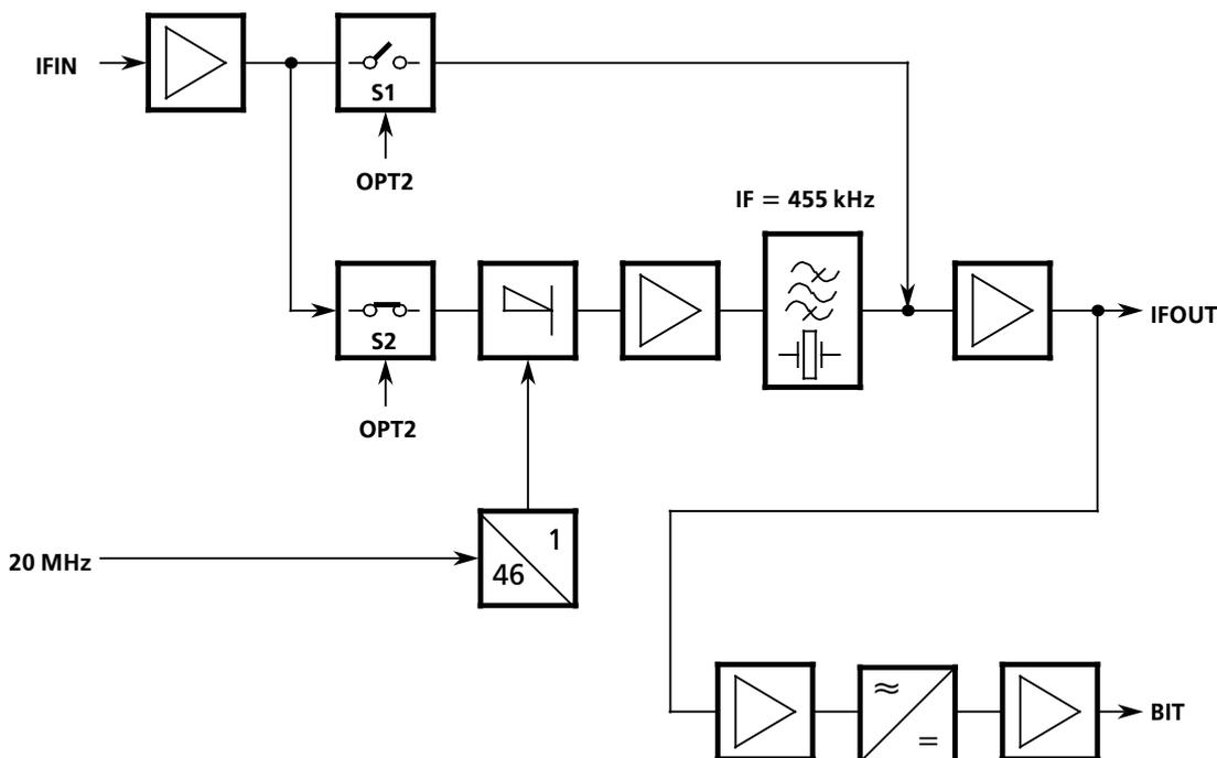
Fig. 1.17 IF Converter R&S UX 895 (Option), Block Diagram
