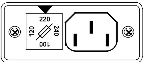
4. For the desired operating voltage insert respective fuse into the fuse holder.
