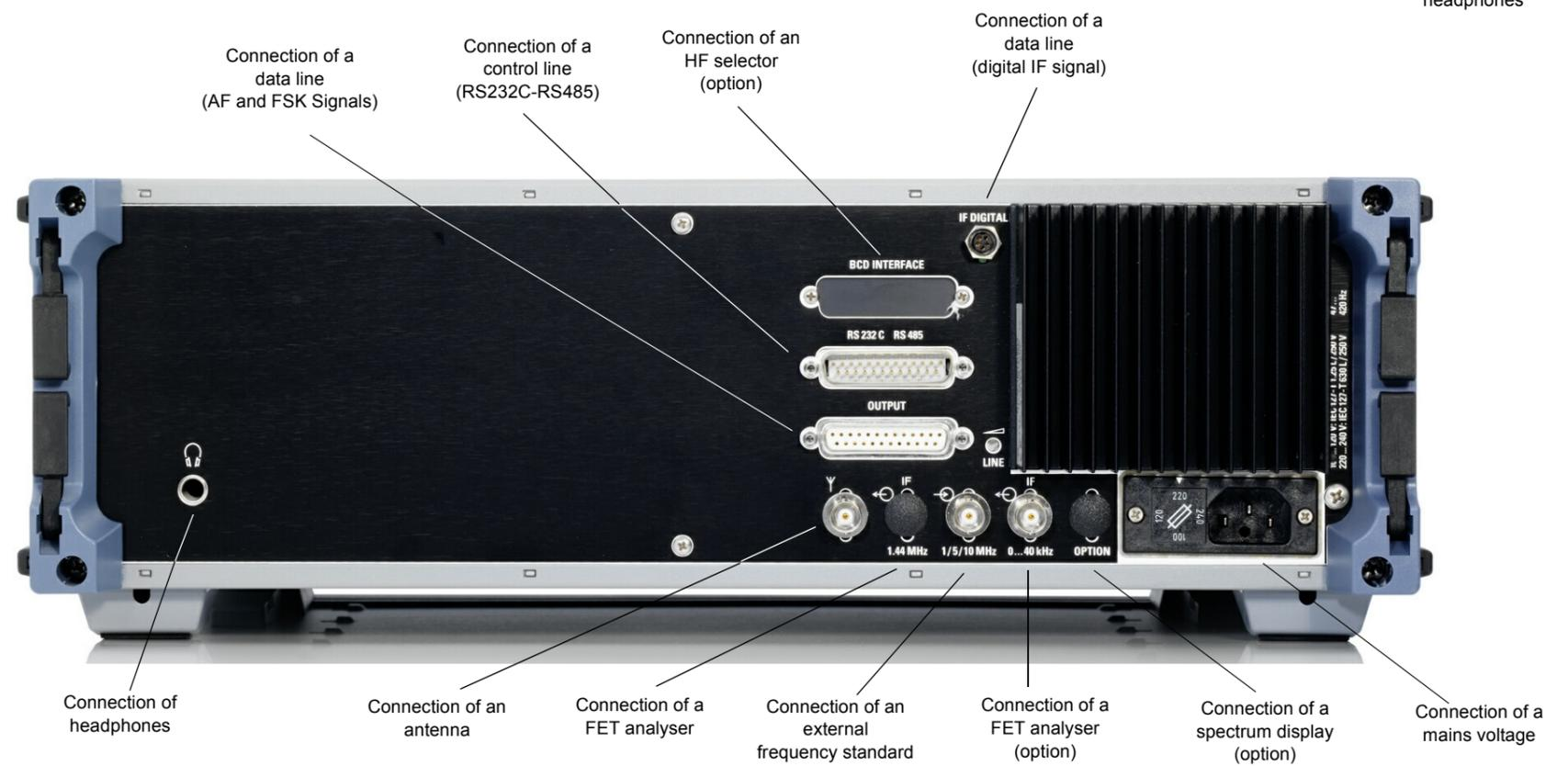
Fig. A2.3 Location of External Interfaces (R&S EK 896)
