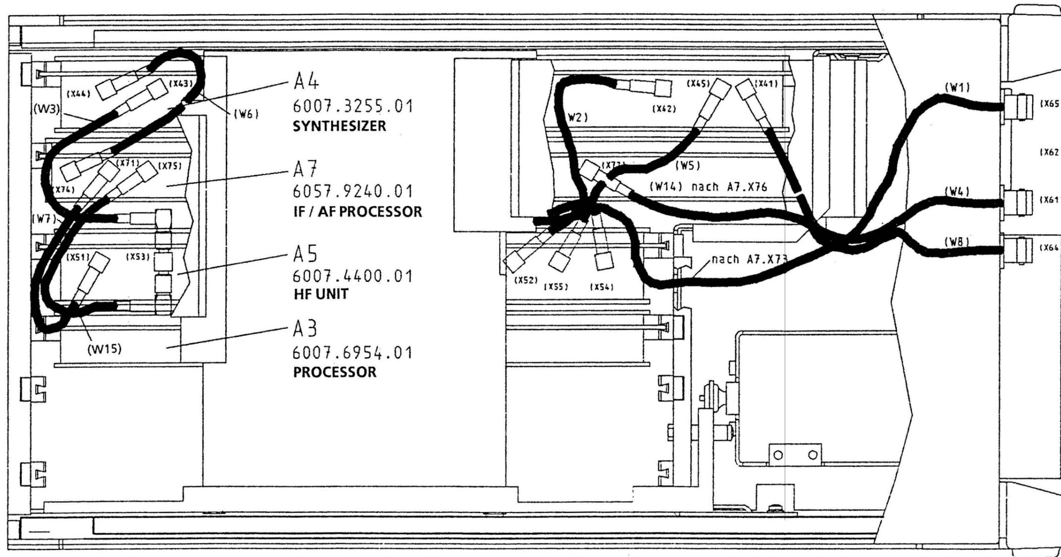
Fig. 4.14 Internal Cabling
