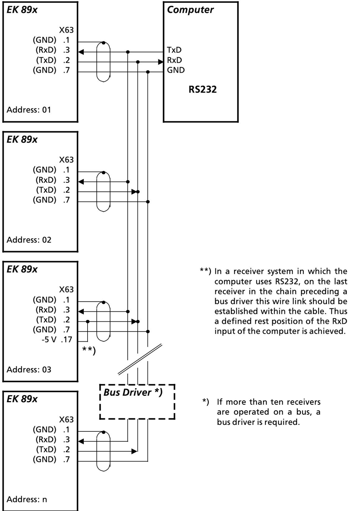
Fig. 2.20 Operating Mode: Four-wire Bus (RS232) with XON-XOFF Handshake (S4 = E or F; see A1.4)
