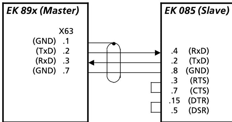
**Fig. 2.18 Operating Mode: RS232 with XON-XOFF Handshake, Master / Slave Operation (S4 = 0 or 1; see A1.4)**
