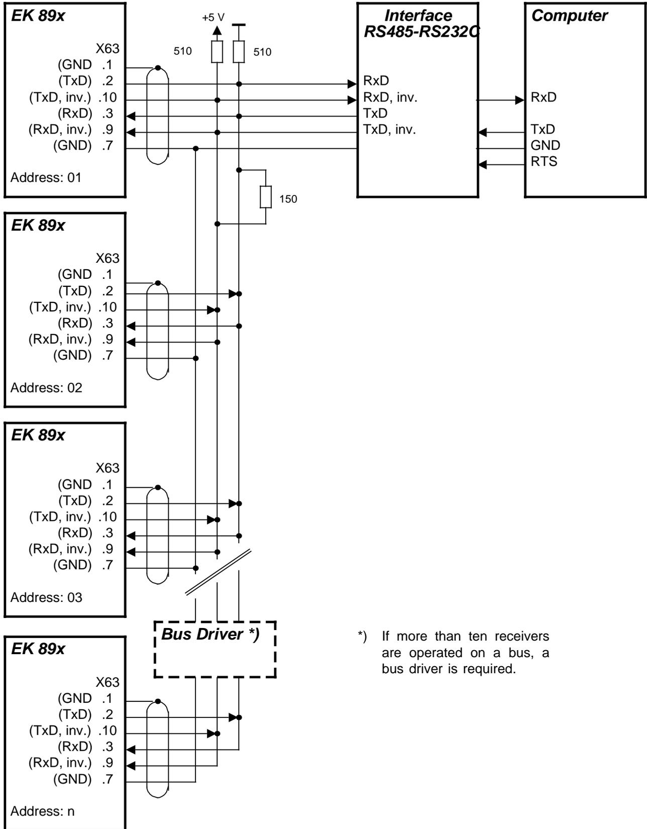
Fig. 2.22 Operating Mode: Two-wire Bus (RS485) with XON-XOFF Handshake (S4 = 8, 9, A or B; see A1.4)
