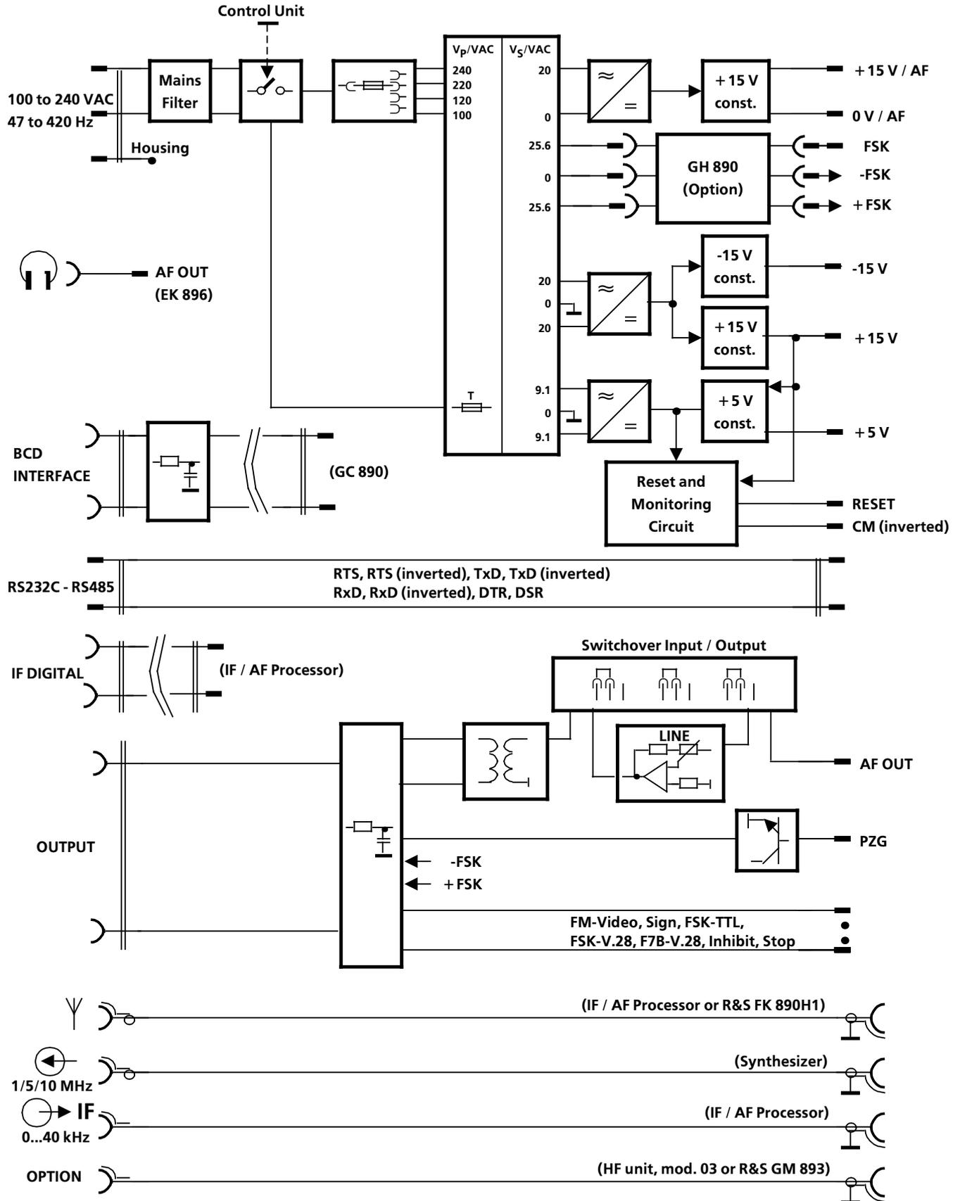
**Fig. 1.11 Power Supply, Block Diagram**
