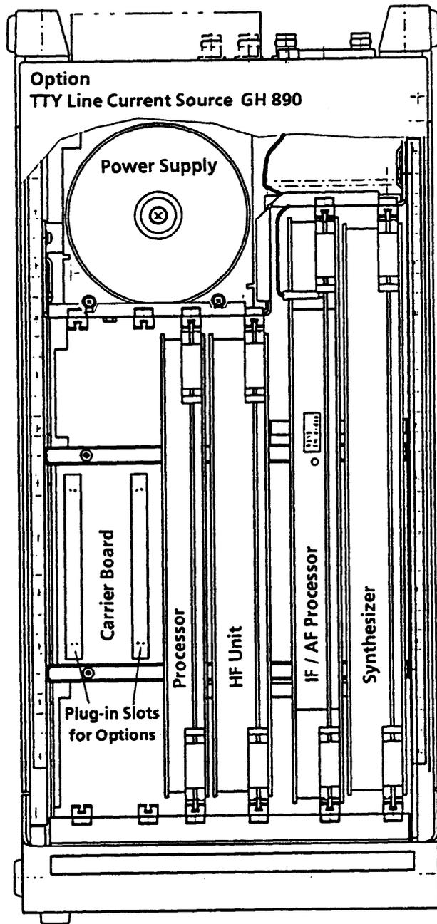
Fig. 1.2 Design of VLF-HF Receiver R&S EK 895
