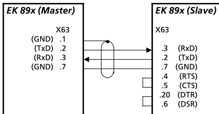
**Fig. 2.19 Operating Mode: RS232 with XON-XOFF Handshake, Master / Slave Operation (S4 = 0 or 1; see A1.4)**
