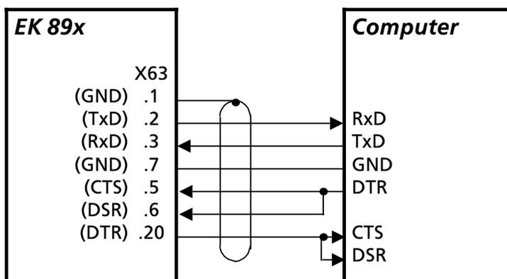
Fig. 2.15 Operating Mode: RS232 with CTS-RTS Handshake (S4 = 0 or 1; see A1.4)
