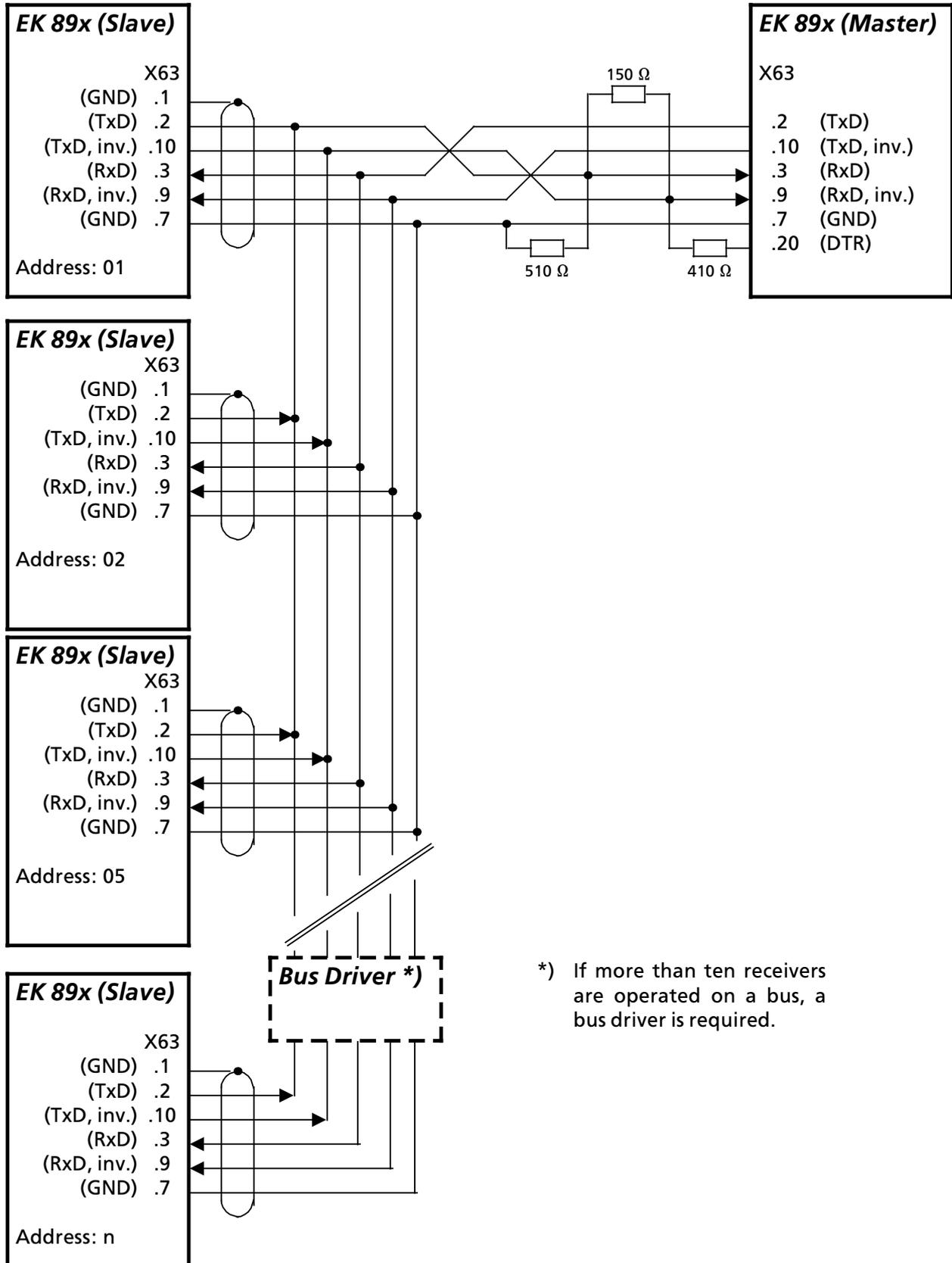
\*) If more than ten receivers are operated on a bus, a bus driver is required.
