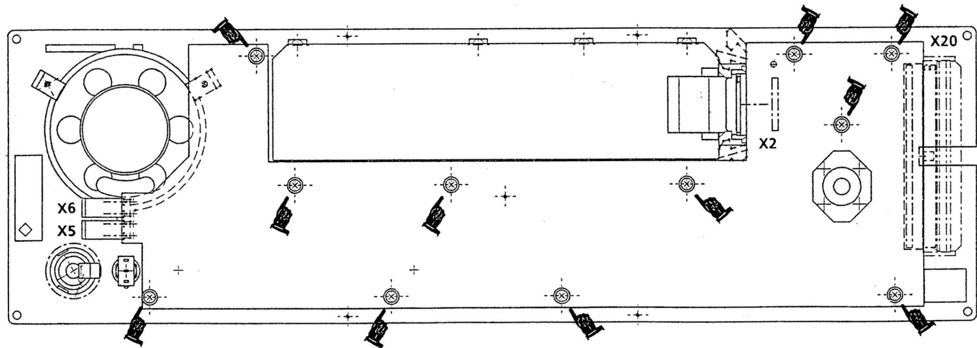
Fig. A1.11 Removal of Control Unit (R&S EK 896 only)
