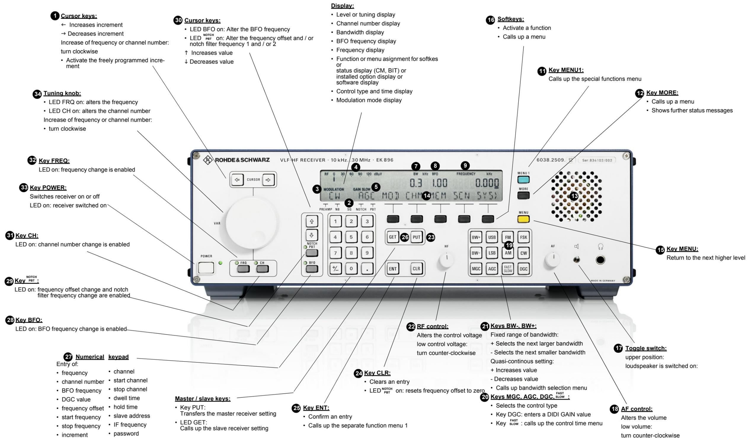
Fig. 3.1 Control and Display Elements of VLF-HF Receivers R&S EK 896
