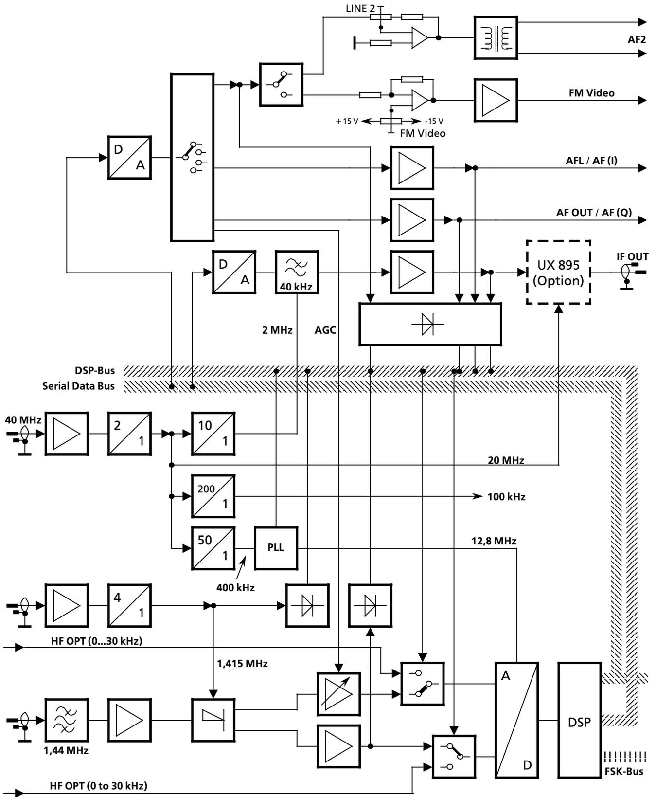
Fig. 1.12 IF / AF Processor Block Diagram
