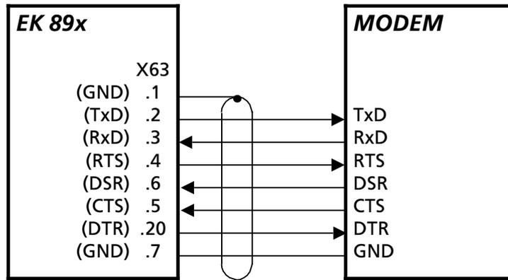
**Fig. 2.17 Operating Mode: RS232 with CTS-RTS Handshake, Asynchronous (S4 = 0 or 1; see A1.4)**
