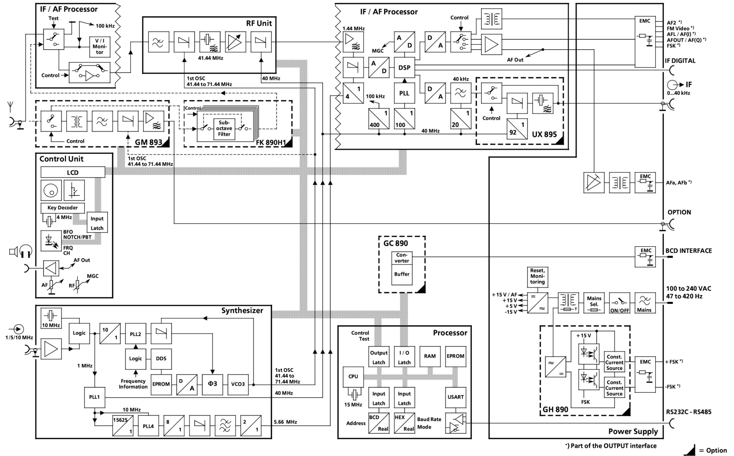
Fig. 1.20 VLF-HF Receivers R&S EK 895, Block Diagram
