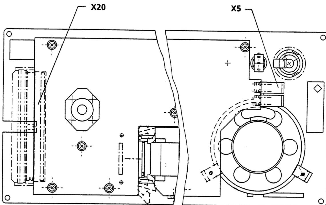
**Fig. 4.4 Location of Connectors X5 and X20 (Control Unit)**
