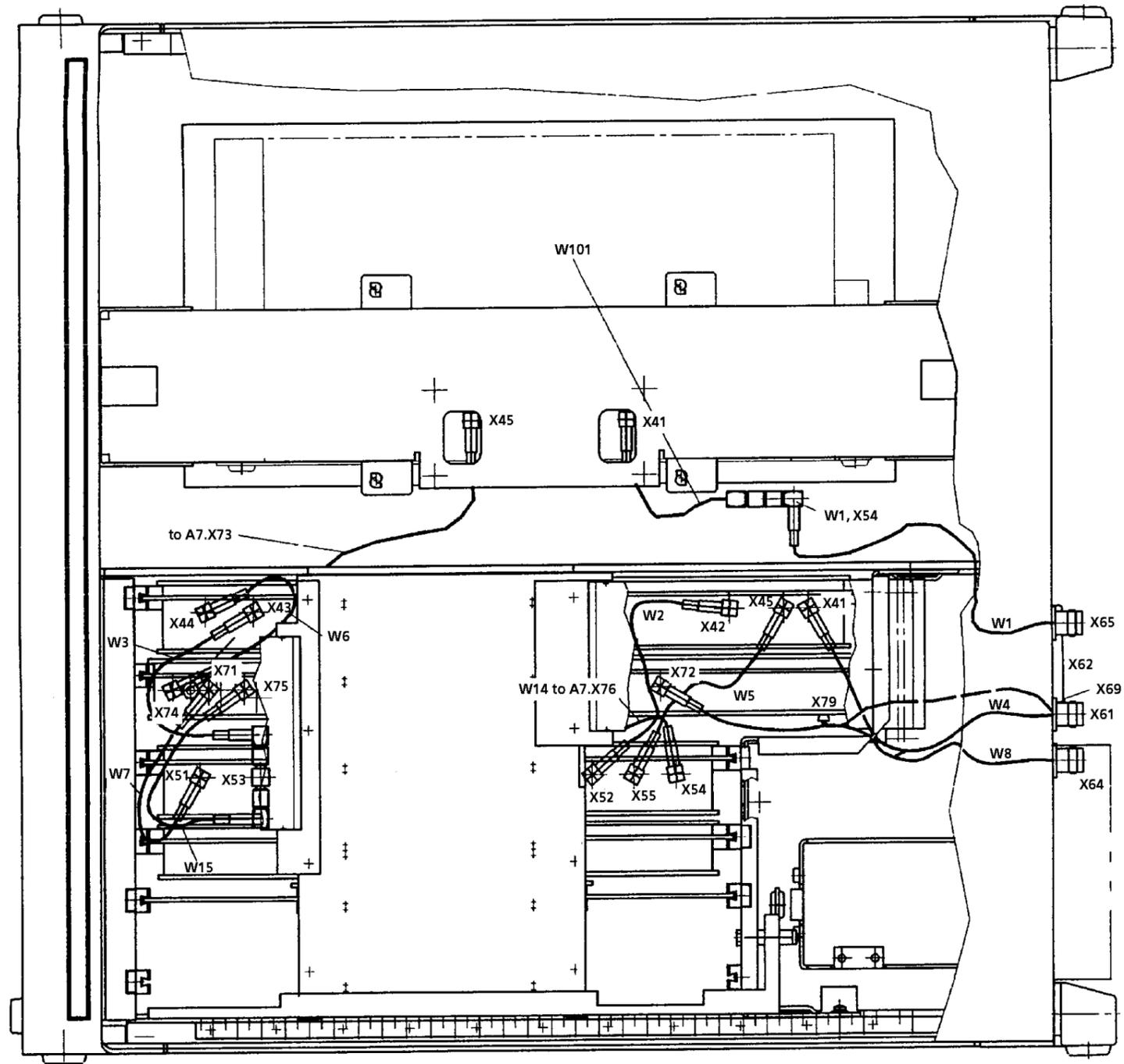
Fig. 4.17 Cabling of VLF-HF Receiver R&S EK 896 with Digitally Tuned RF Selector R&S FK 896D
