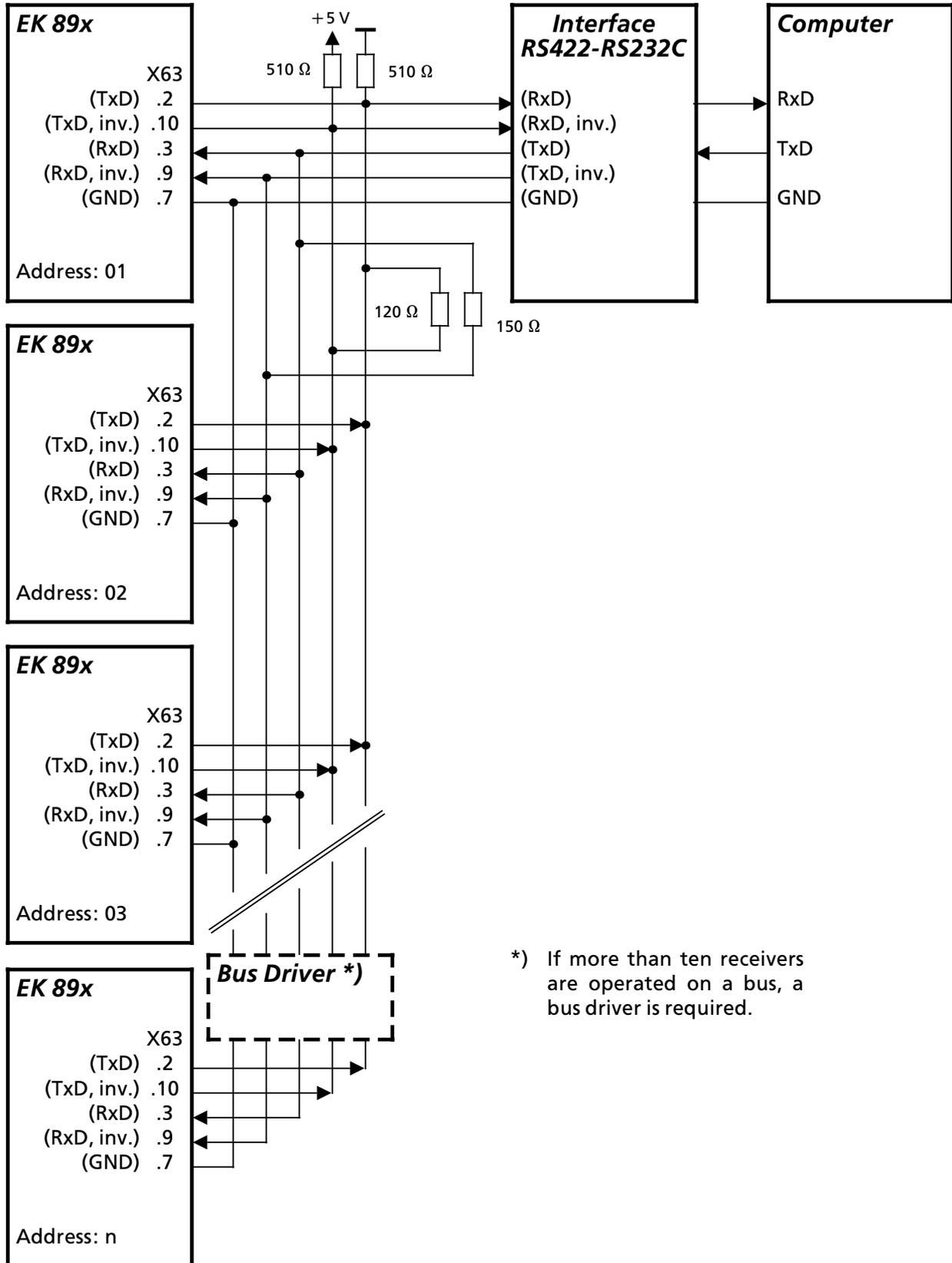
Fig. 2.21 Operating Mode: Four-wire Bus (RS485) with XON-XOFF Handshake (S4 = E or F; see A1.4)
