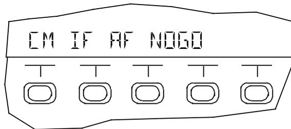
or both synthesizer and IF / AF processor defective
