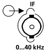
Connect the recessed BNC socket via an RF cable to an analyzing device (e.g. analyzer FET).
