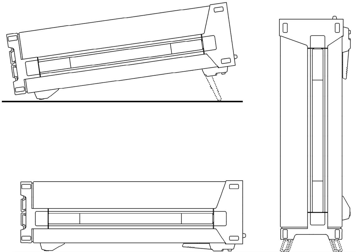
**Fig. 2.1 Possible Positions for Installation**
