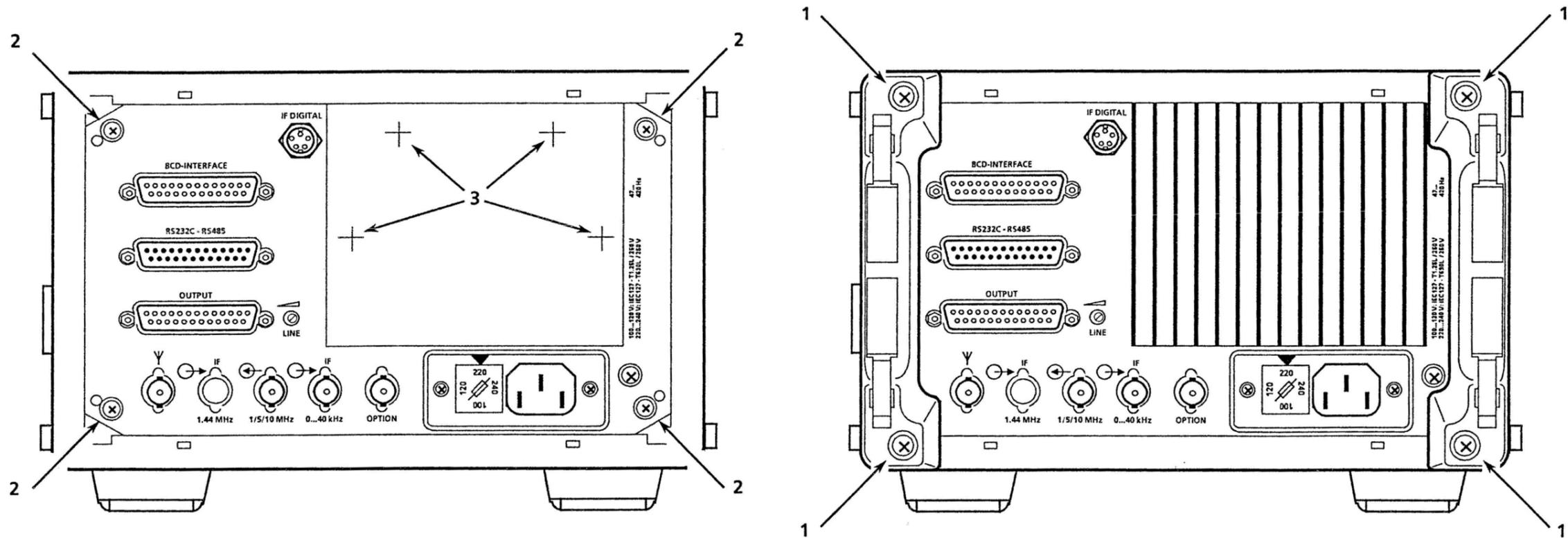
Fig. 4.10 Location of Screws to Be Undone On Front (R&S EK 895)
