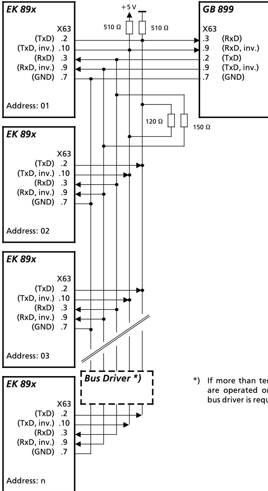
\*) If more than ten receivers are operated on a bus, a bus driver is required.
