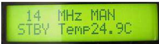
This mode is for AC Power ON, and OPER. Switch at STBY position. Amplifier is in a through state.
