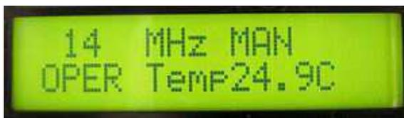
This mode is for AC Power ON, and OPER switch at OPER. Position. Amplifier will work, if the transceiver is keyed.
