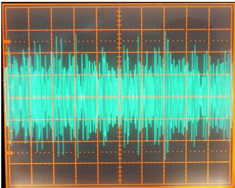
12. **Subjective TX audio test:** In this test, a headset is plugged into the microphone and headphone jacks and a transmitted SSB signal is monitored with MON active.
