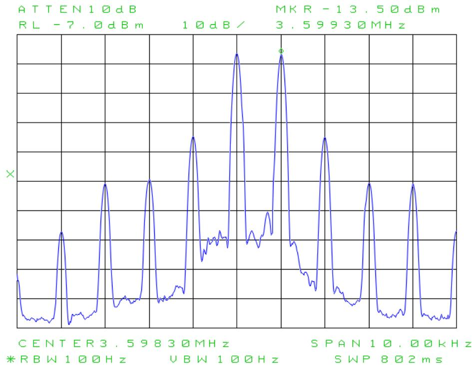
Figure 8: Spectral display of 2-tone IMD at 14.1 MHz, 200W & 50W PEP.
