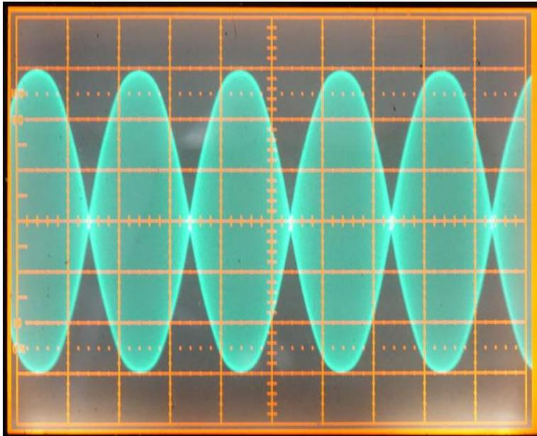
11. **ALC Overshoot Test with White Noise.** In this test, white noise is applied applied to A ACC1 Pin 4 (MOD IN) from an HP 8935 test set. The terminated oscilloscope is connected to ANT1 via a 50 dB high-power attenuator.
