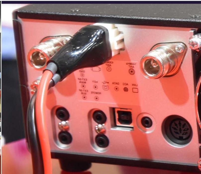
You can see connectors on the rear panel through the display back mirror. There are several connectors for LAN, DATA, USB and REMOTE.
