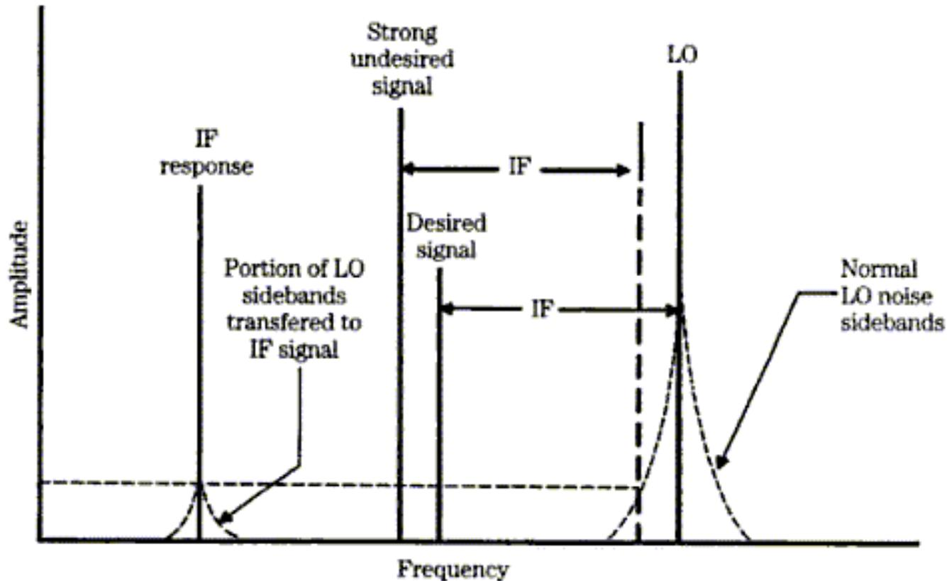
Reciprocal mixing noise can degrade and even completely mask a weak desired signal.
