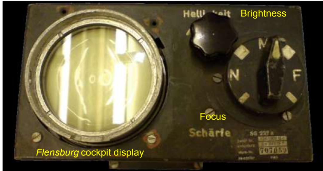
*Flensburg* was a threat receiver fitted to Luftwaffe night-fighters in Spring 1944, and tuned to the 300 MHz emissions of the RAF *Monica* tail-warning radar. It had good sensitivity and angular discrimination, and enabled the fighter pilot to pick out a single bomber even in a stream, radiating multiple *Monica* signals.
