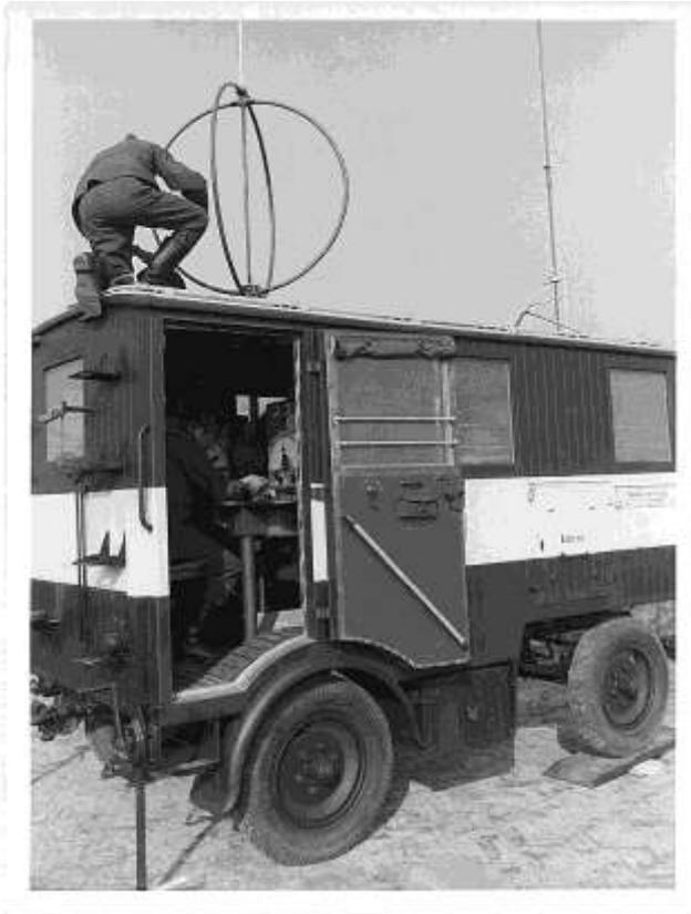
**Left: D/F antenna. Right: HF TX antenna.**
