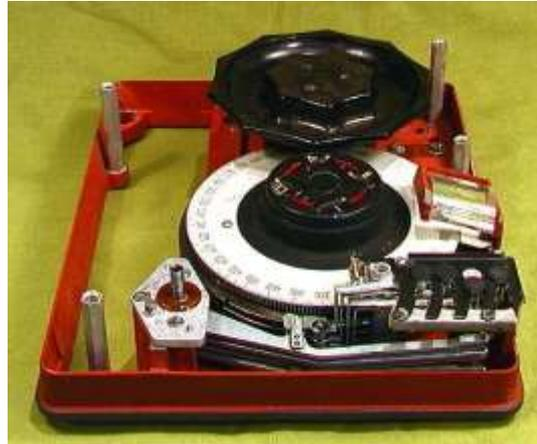
**EK** front panel frame & tuning dial mechanism with 4 preset cams.
