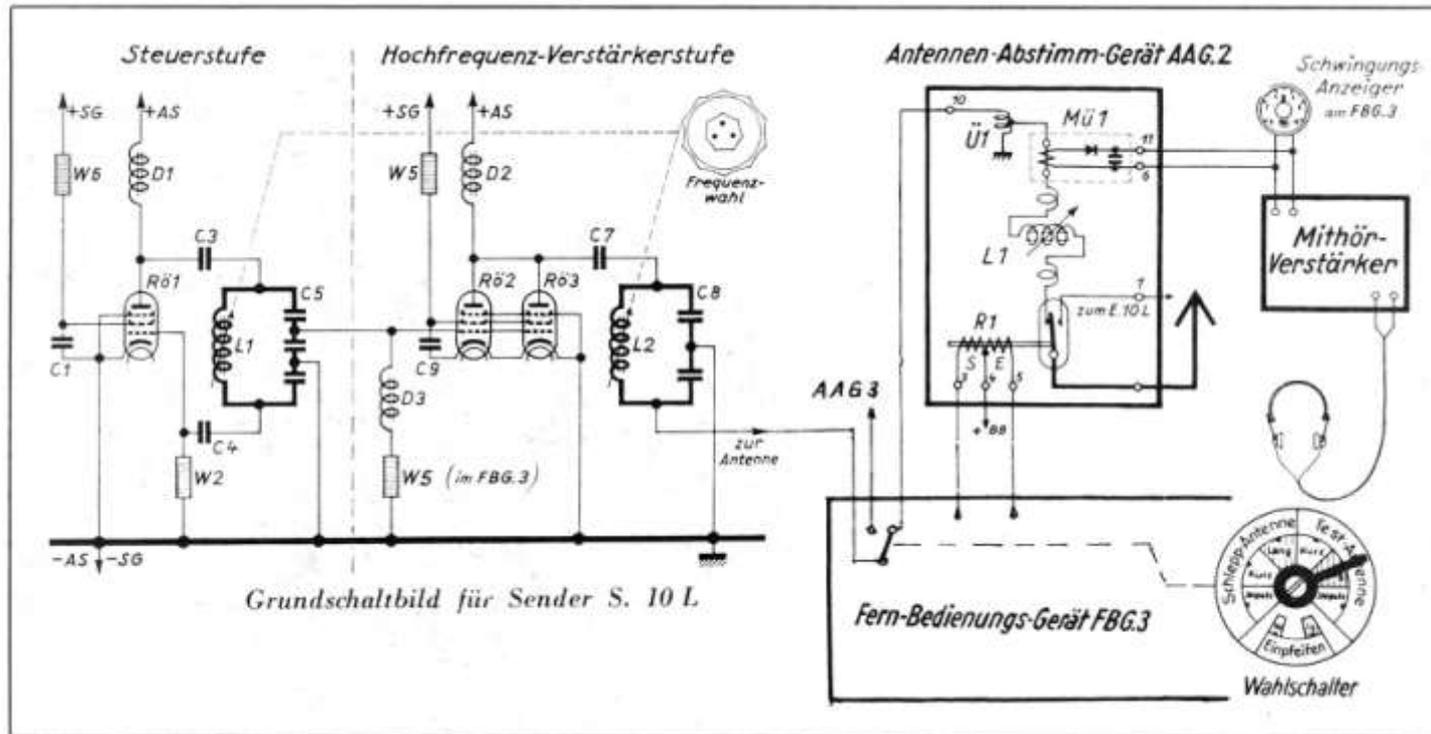
Note 1: Connections from TX and RX via Ant. Control Unit (FBG.3) to ATU (AAG.2) are 60Ω coax.
