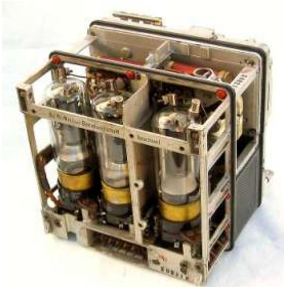
**SK Transmitter** with RL12P35 tubes
