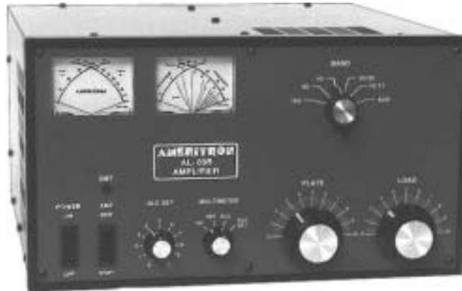
1. Power up and select desired band. Select CW at exciter. Note  $I_{p0}$ .
