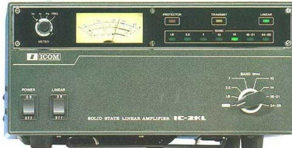
1. Power up. Set **METER** switch to **PRO** (ALC CAL). Select CW at exciter. Set **ALC** pot (on rear panel) to minimum. Set **BAND** to AUTO (assuming Icom exciter).
