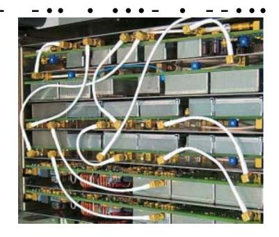
RF packaging is built to the highest industrial standard: completely shielded modules with 50Ω SMB coax connectors, mounted on FR4/G10 PCB cards. Note Teflon® coax jumpers.
