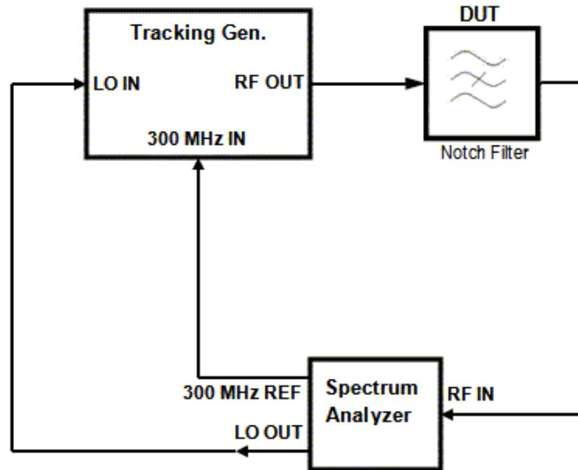
Fig.9: Block diagram of 2-port scalar network analysis setup.
