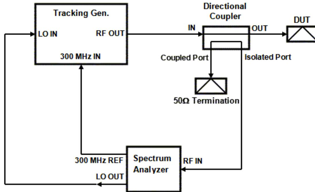
Fig.12: Block diagram of 1-port scalar network analysis setup.
