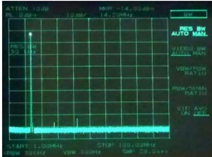
Fig.4: Harmonics/spurs display.
