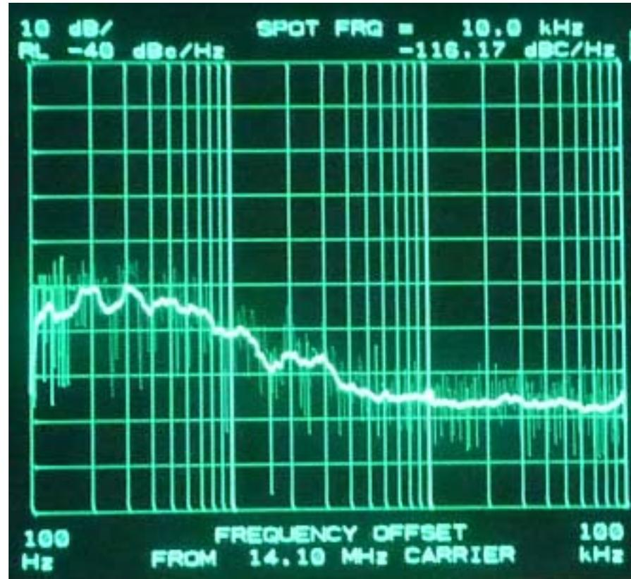
Fig.6: Phase noise test results (HP 85671A phase-noise utility).
