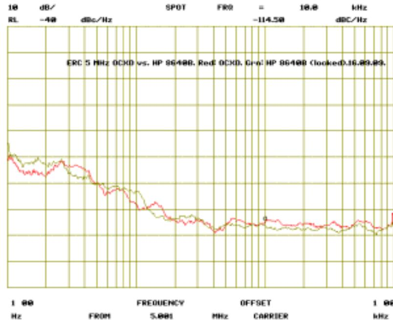
Fig.7: Phase noise of precision 5 MHz OCXO vs. HP 8640B sig. gen.
