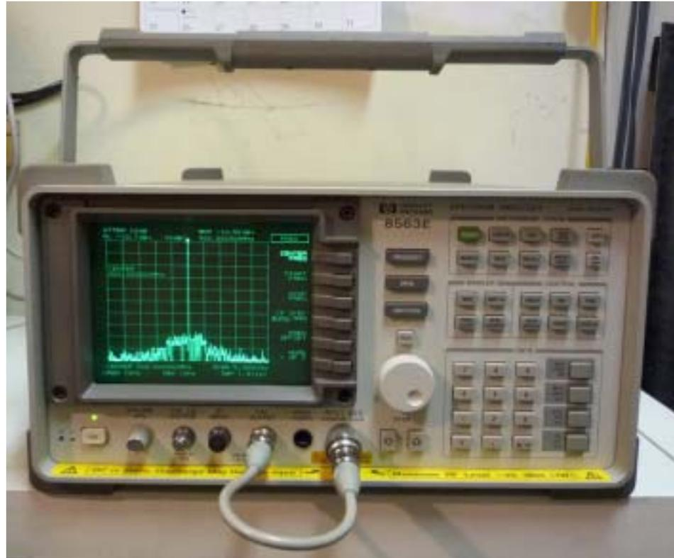
Fig.1: HP 8563E Spectrum Analyzer with HP 85620A Mass Memory Module.
