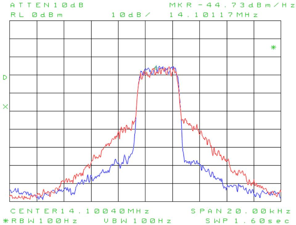
**Figure 4a: White Noise IMD at 14.1 MHz, 100W PEP, PureSignal (PS) off & on (Test 9a, 50 kHz).**
