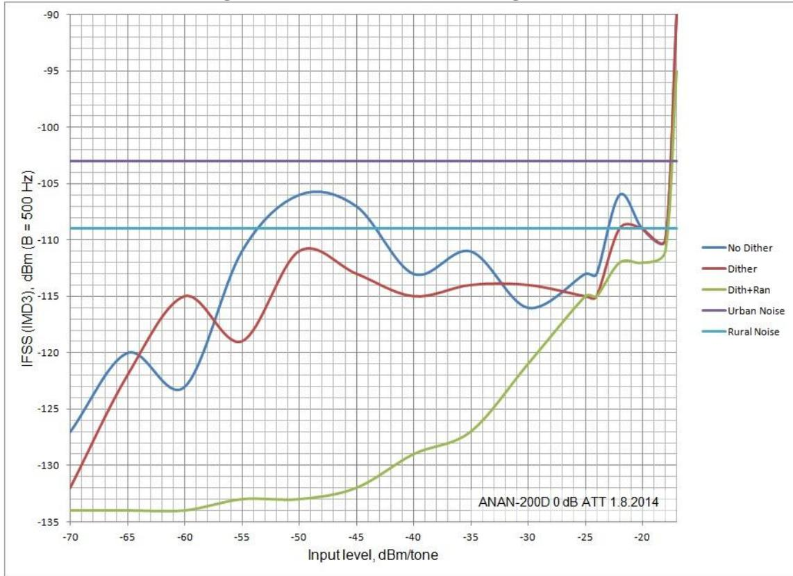
**Note on 2-tone  $IMD_3$  test:** A comparison between the above chart and that for the ANAN-100 (main report, Figure 5) will be of interest. In the ANAN-200D, the reduction in  $IMD_3$  product levels with increasing input level is greater than in the ANAN-100D, especially in the -58 to -40 dBm input level range, although the ANAN-100D exhibits lower  $IMD_3$  levels over a wider input power range than the ANAN-200D.
