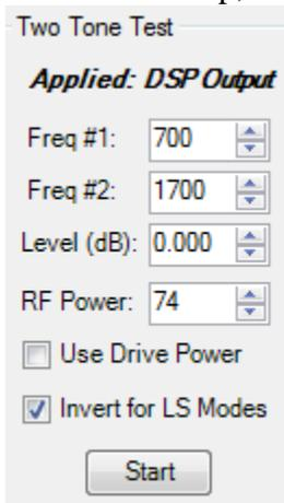
2. Click **Start** and adjust RF Power for 100W PEP (-16 dBm per tone) on spectrum analyzer. Click **Start** again to stop transmitting.
