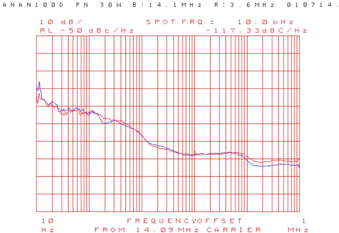
**Figure 20b: Composite noise at 50.1 and 14.1MHz, 30W.**
