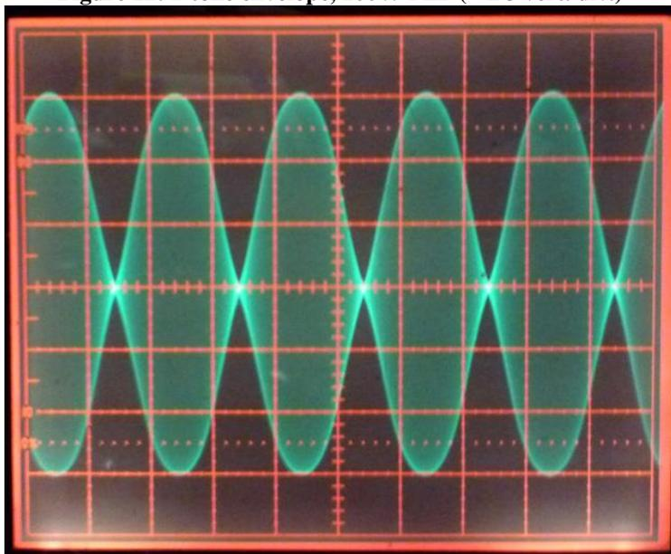
**16a: Subjective TX audio test:** In this test, a headset is plugged into the microphone and headphone jacks and a transmitted SSB signal is monitored with MON active.
