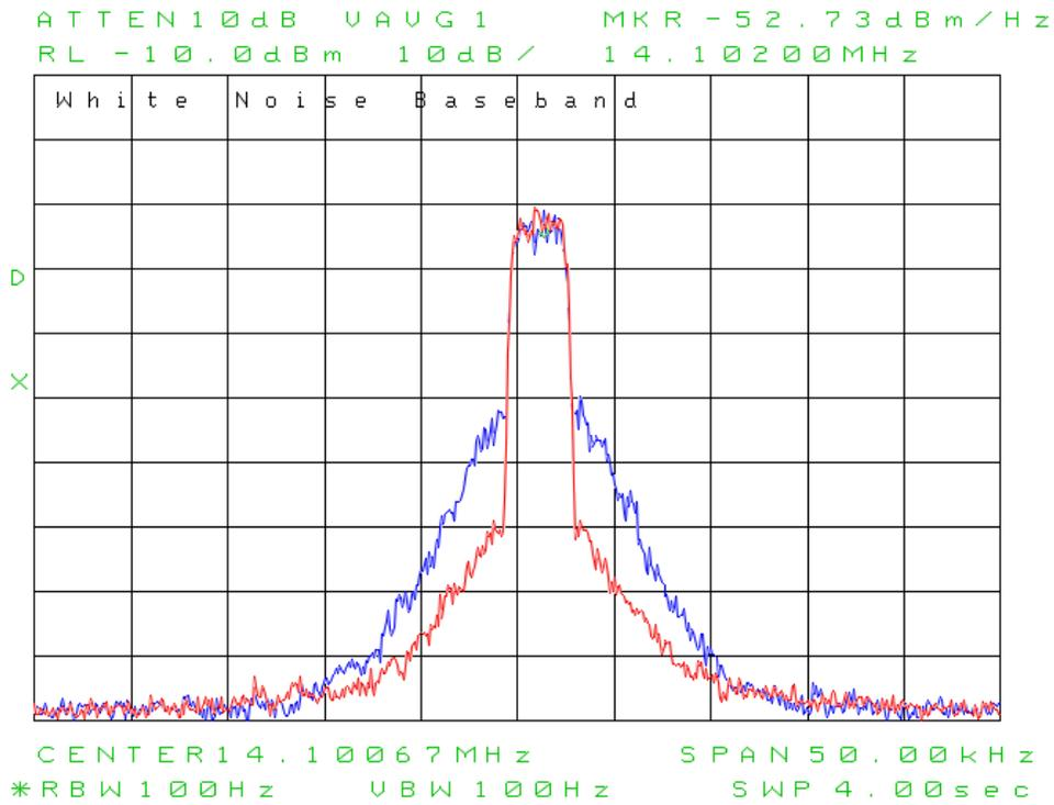
**Figure 5: TX composite noise at 14.1 MHz, 30W.**
