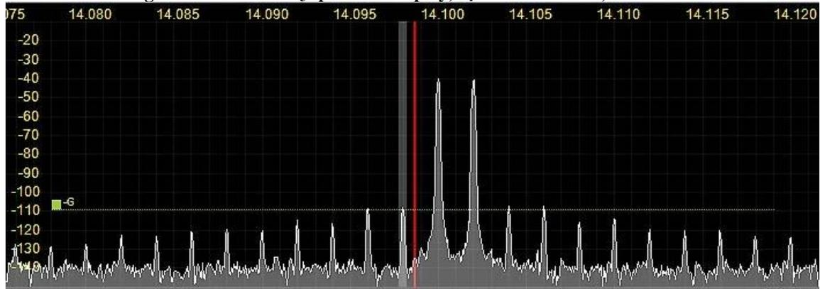
**9. Two-Tone 2<sup>nd</sup>-Order Dynamic Range (DR<sub>2</sub>).** The purpose of this test is to determine the range of signals far removed from an amateur band which the receiver can tolerate while essentially generating no spurious responses within the amateur band.
