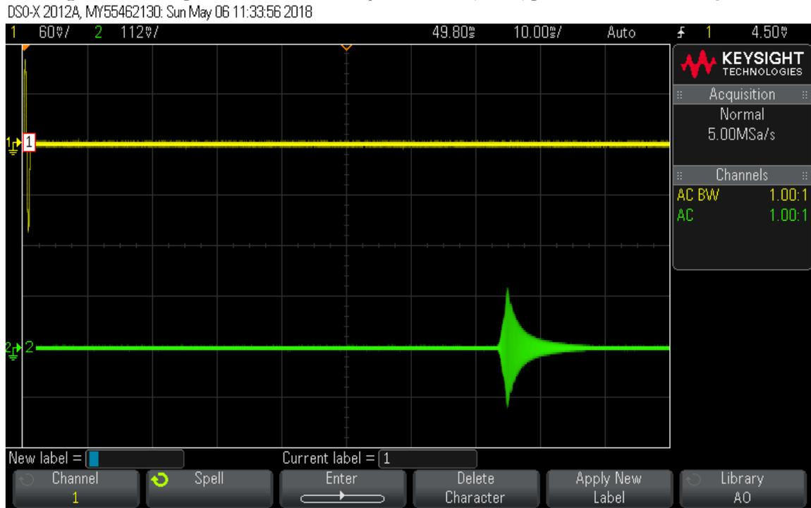
**Figure 40: Example of 2-tone latency test: all OFF.**
