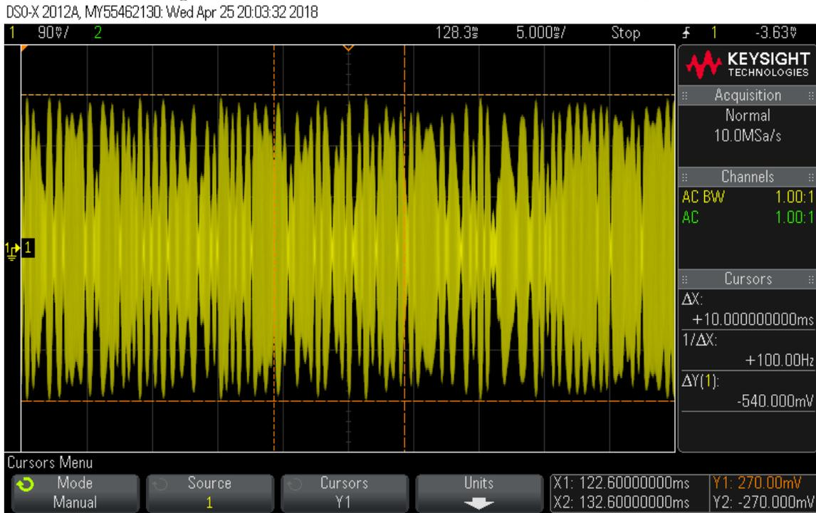
**21: ALC Compression Check.** In this test, a 2-tone test signal is applied to the USB port from the internal 2-tone generator. An oscilloscope is connected to the DUT RF output via a 50 dB power attenuator. RF Power is initially adjusted for 100W CW output.
