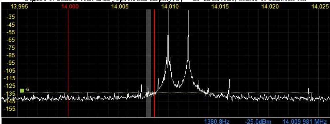
**10: Two-Tone 2<sup>nd</sup>-Order Dynamic Range (DR<sub>2</sub>).** The purpose of this test is to determine the range of signals far removed from an amateur band which the receiver can tolerate while essentially generating no spurious responses within the amateur band.
