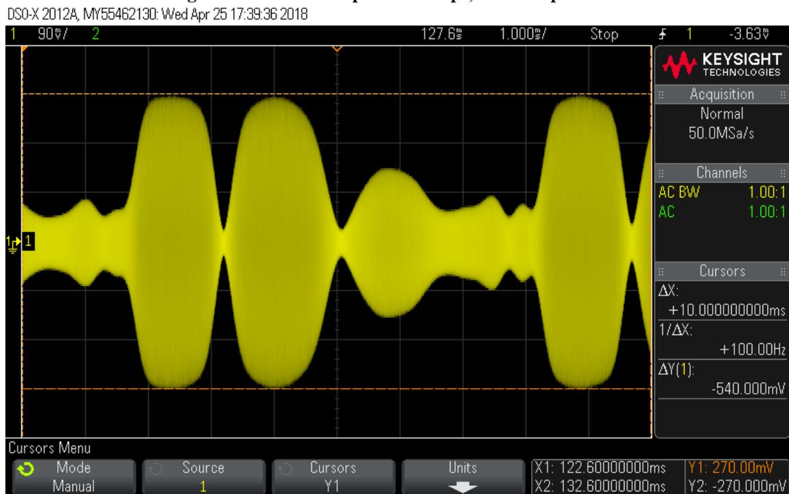
**Figure 14: 100W speech envelope, 10dB compression, CESSB off.**
