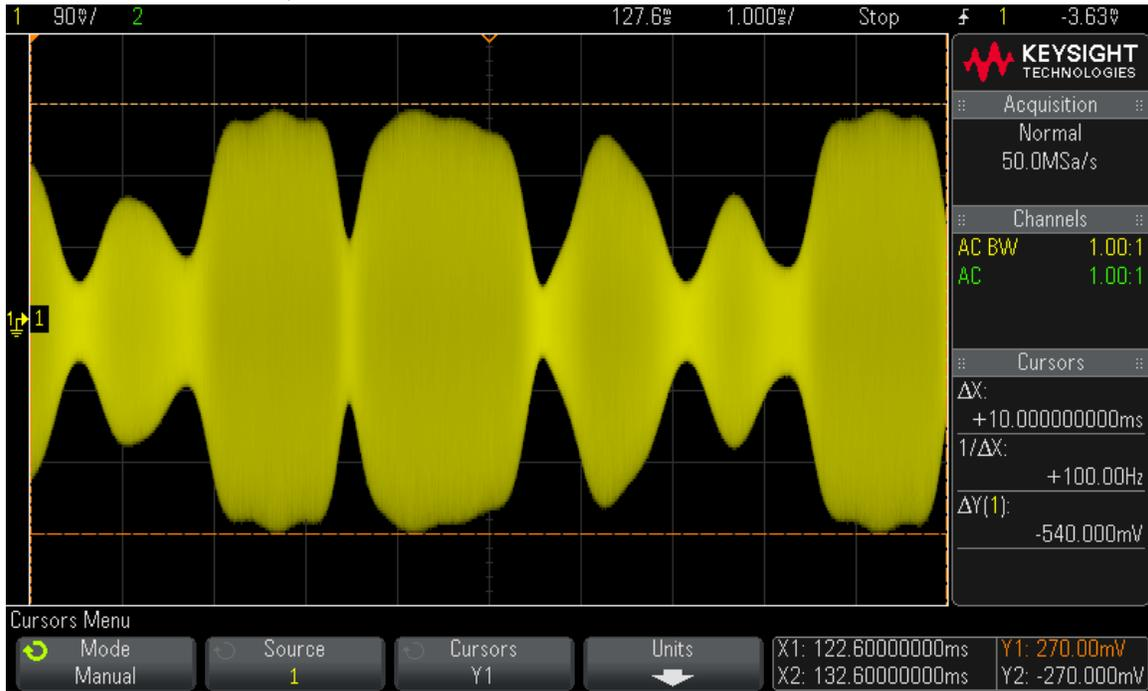
**Figure 15: 100W speech envelope, 10dB compression, CESSB on.**
