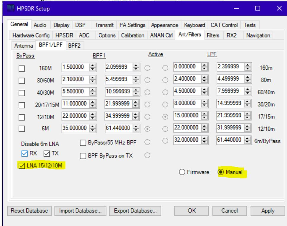
The options were configured as per Figure 31, and MDS measured using an RF signal generator connected to ANT1 and an RMS AC voltmeter connected to the HEADPHONE jack. Test results are given in Table 15.
