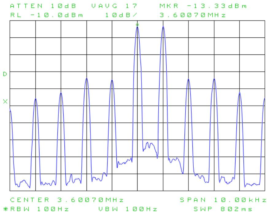
**Figure 14: Spectral display of 2-tone IMD at 14.1 MHz, 200W**
