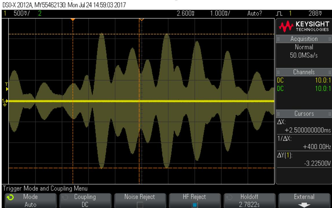
**Figure 33: Transmitted RF envelope, USB, 200WPEP, CFC on, VA7OJ Test profile.**
