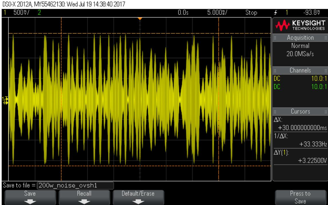
**20: ALC Compression Check.** In this test, a 2-tone test signal is applied to the USB port from the internal 2-tone generator. An oscilloscope is connected to the DUT RF output via a 60 dB power attenuator. RF Power is initially adjusted for 200W CW output.
