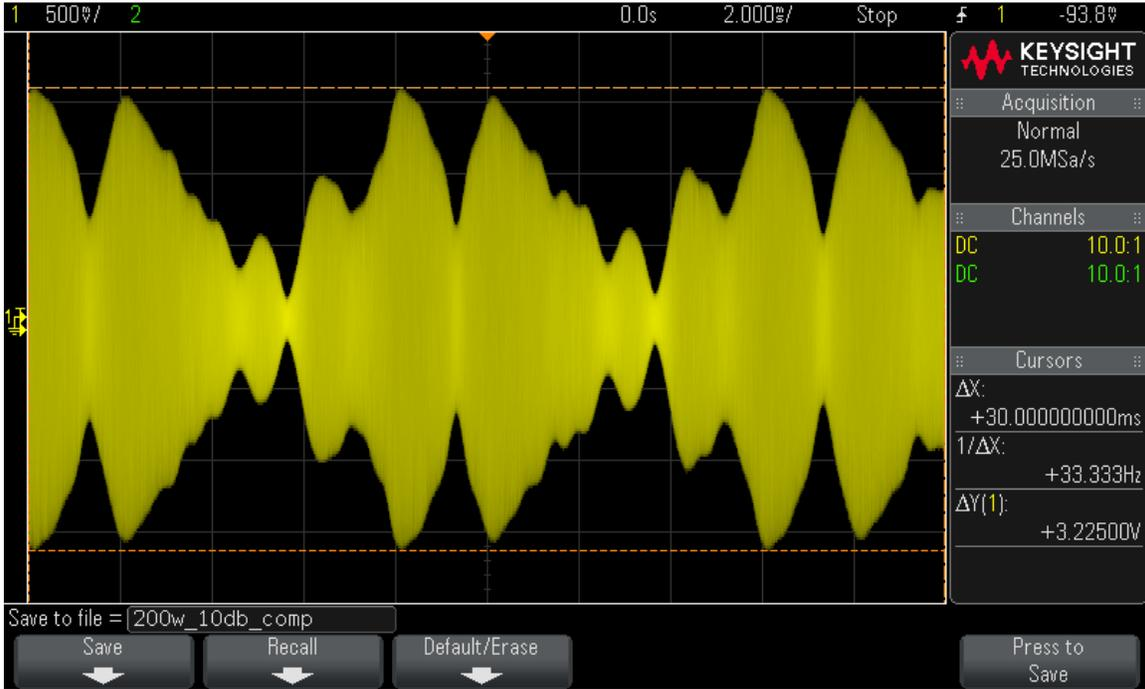
**Figure 10: 200W speech envelope, 10dB compression, CESSB on.**
