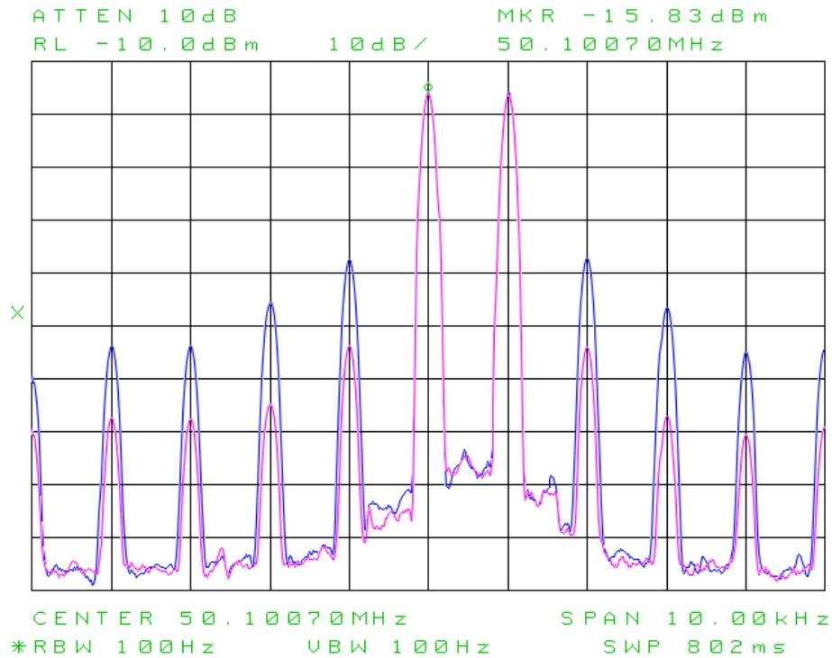
**Figure 29: AM Sidebands for 90% Modulation, PureSignal on. THD  $\approx$  0.25%.**
