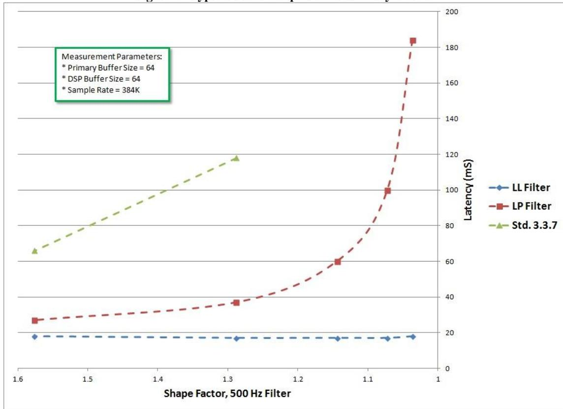
**Note:** LL: V3.3.9.0 (released June 2016) and all subsequent builds incorporate the LL (Low Latency) and LP (Linear Phase) filter options.
