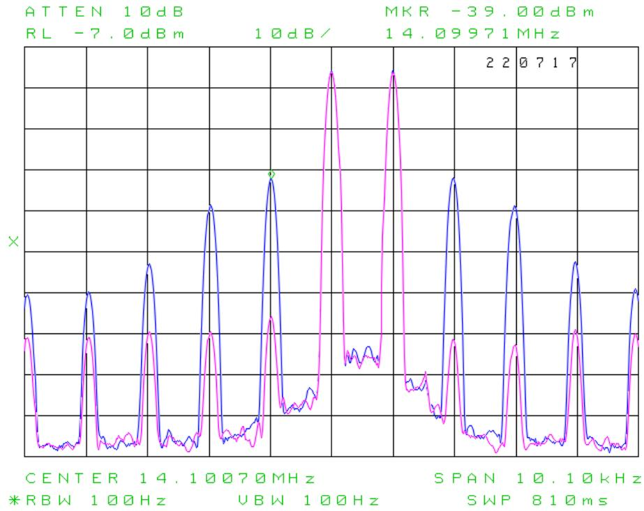
**Figure 28: 2-tone TX IMD at 50.1 MHz, 100W PEP, PureSignal (PS) off & on.**
