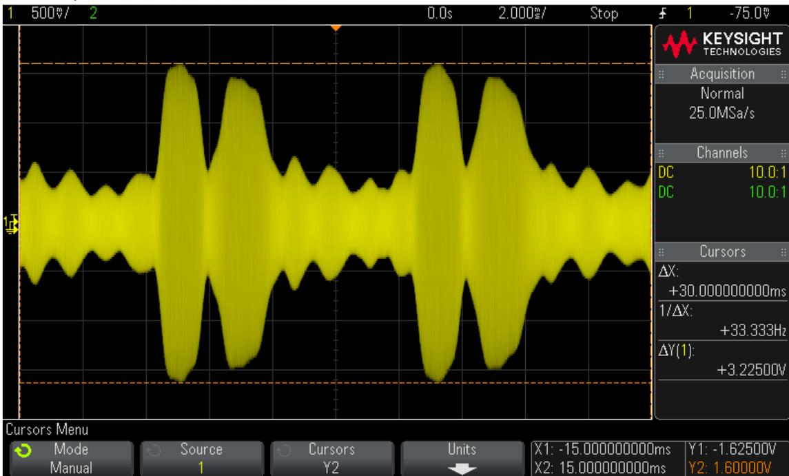
**Figure 9: 200W speech envelope, 10dB compression, CESSB off.**
