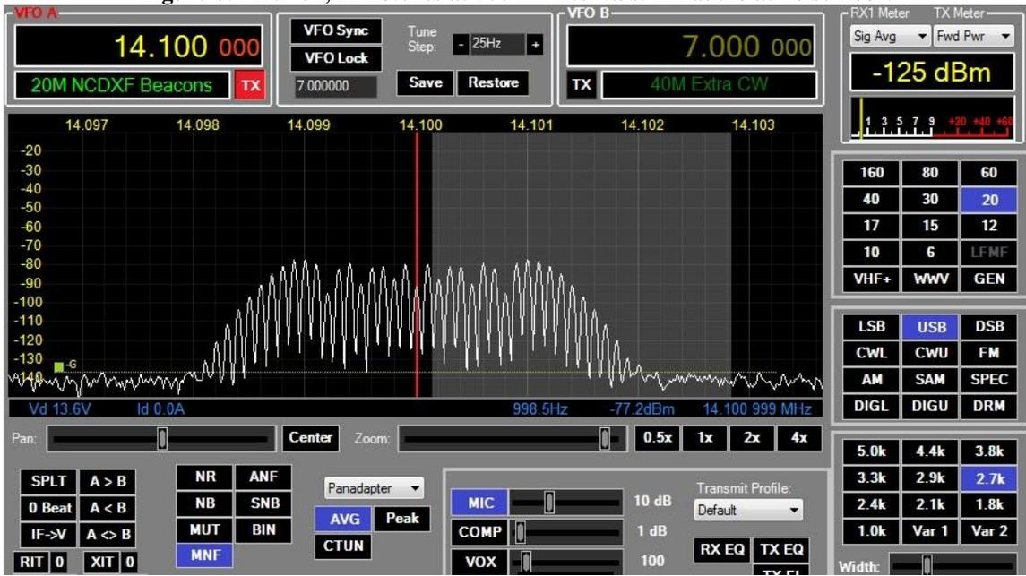
**7: AGC impulse response.** The purpose of this test is to determine the Anan-8000DLE's AGC response in the presence of fast-rising impulsive RF events. Pulse trains with short rise times are applied to the receiver input.
