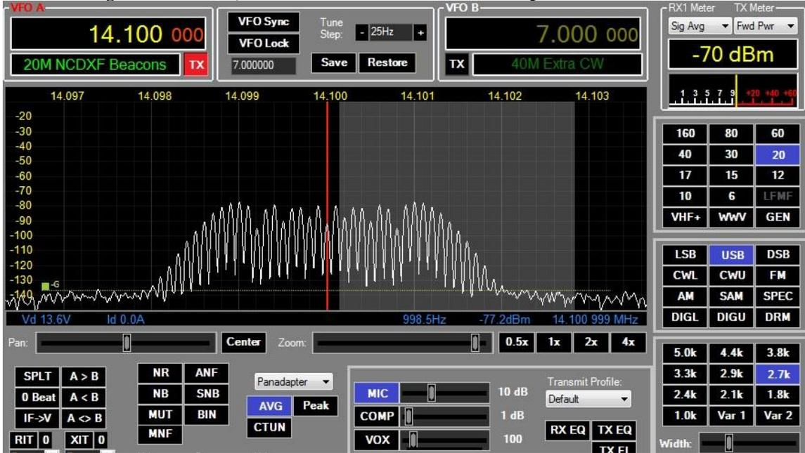
**Figure 6: MNF on, 21 notches at 100 Hz intervals. RX audio at noise floor.**
