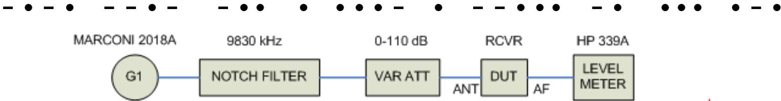
BLOCK DIAGRAM OF RECIPROCAL MIXING TEST SETUP
