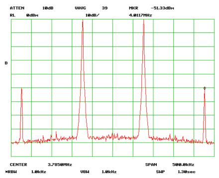
4. Noise Figure(NF): NF was measured by the "modified Y-Factor" method, using the following test setup: NoiseCom NC6110 noise generator ▶ 0-110 dB step attenuator ▶ MCL BLP-30 30 MHz LPF MCL FT1.5-1B 50/75Ω transformer ▶ DUT ▶ MCL FT1.5-1C 75/50Ω transformer ▶ MCL GALI-74\* wideband amplifier ▶ 2 dB pad ▶ HP 8563E spectrum analyser. V<sub>CC</sub> was +13.8V.
