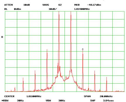
DXE-RPA-1 Preamp (VE7KW). Actual output +15 dBm/tone. 150 kHz spacing. 03.10.2013.
