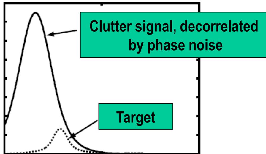
High phase noise in radar LO spreads clutter signal and masks desired low-level target response
