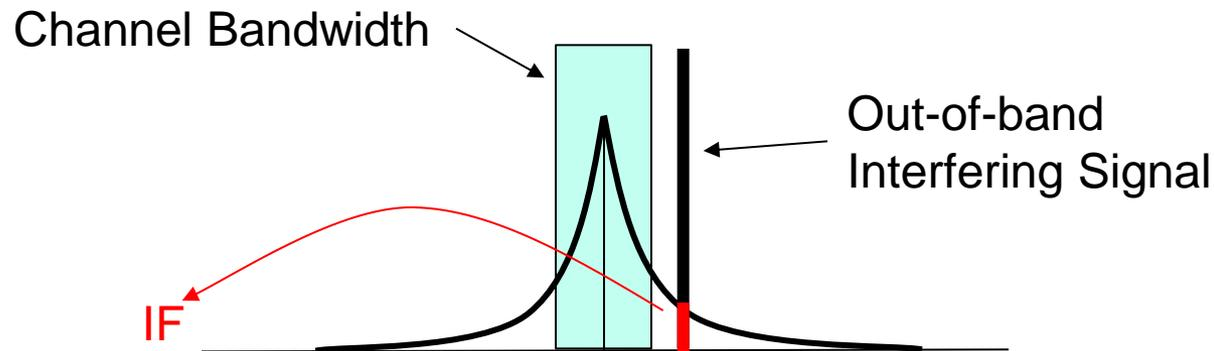
Large interferer mixes with LO energy spread by phase noise to produce a signal in the receiver IF – reduced sensitivity
