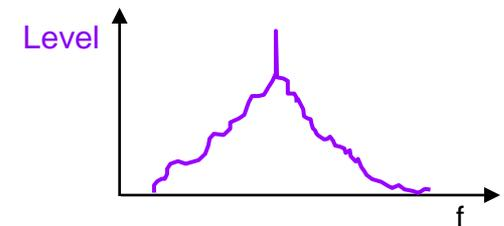
**Phase Noise is unintentional phase modulation that spreads the signal spectrum in the frequency domain.**
